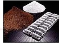
Red Bauxite, white alumina, and silvery aluminium
