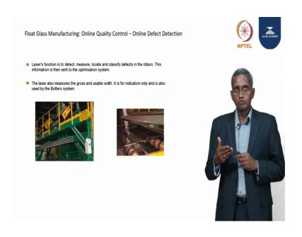
Online we also have all the float lines are equipped with a any high tech deduction devices which can spot defects. Un-melted raw materials or bubbles which come because of a pure refining which we talked about the CO 2 that has to escape out of the glass if not done efficiently it can pass into the glass.
