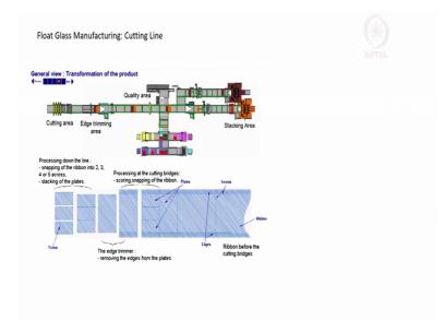
And thus you can see you can cut it into a big size glass called as a jumbo glass or you can cut into medium sized glasses which is called as a DLF or the small standard size is
