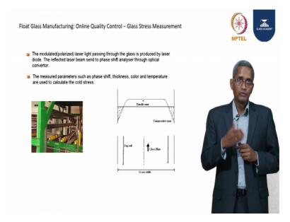
And next is we talked about the stress profile. On the annealing Lehr and there are online equipments which measure and tell us continuously how much is the stress on the glass, so that we can regulate and avoid bad stress glass being sent to the customer.
