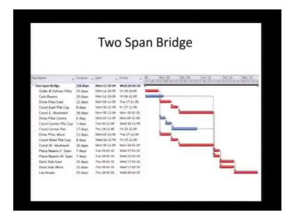
We are taking we are going to take just the concreting crew the piling crew and the bridge lunching crew and here is the bar chart of the two span bridge and if you recall this is with unlimited resources we have put it on to a project planning software. So, you will start slowly getting introduced to the project planning software tool, and you remember we had 2 critical paths, we had the 2 abutments that were critical the middle was not so critical you can see generally that is here.
