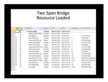
And we are using these resources we are using you know the precasting gang we are using a piling we are using concreting we are using a group of resources for girder launching and road block. So, these are the key resource group, we are going to use.
