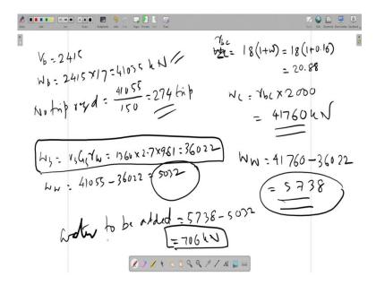
So, let me create another page and then go back to the problem. So, this one so, here actually that your fourth problem was if a dump truck can carry 150 kilo Newton of soil in the trip, what will be the number of trips required to transport the soil to the construction site. So, 150. I have to find out now, what is the total weight of the soil actually we are bringing from the borrow site.
