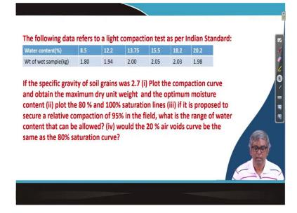
Now, let me go to the next box problem. So, this is the second problem here. We can see this is the problem we have also critically and we have discussed that when you do compaction test in the proctor compaction or modified compaction, there is a mold and that mold will be compacted in a particular standard way and then the weight will be taken and weight of the weight sample that means a compactor mold and what is the water present that data will be collected occasionally in a particular test.
