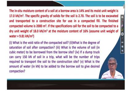
Yes, this is the first problem, you can see the in-situ moisture content of a soil at a borrower area is 14% borrow area from soil will be taken and its moist unit weight is 17 kN/m<sup>3</sup>. The moist unit weight means bulk unit weight, as it is. So, everything 17 kN/m<sup>3</sup>  $\gamma$ -bulk is 17 and water content is 14w equal to 14%.
