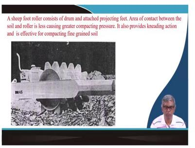
See I have mentioned perhaps one of the roller types that is sheep foot rollers and as you can see here, the sheep foot roller means actually the main roller and on that there is a protruded part and what is the purpose of these actually, when the roller is only passing the roller resting on those extended portion and as a result contract area will be reduced and more pressure can be applied to the soil and at the same time there will be kneading effect.
