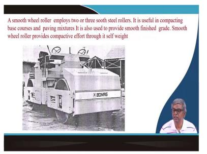
And this is again smooth wheel rollers most of the time finished surface generally smooth wheel rollers or rollers are used. In addition to that compacting base course, are also paving mixtures also can use it is also used to provide smooth finish surface as I mentioned the beginning.
