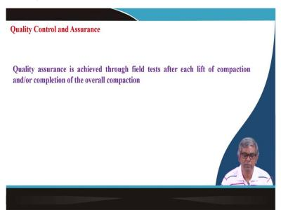
Next part is quality assurance it is achieved through field test after each lift of compaction that means each and every compaction Atterberg's will check, then to the bottom three layers are under compacted and topmost layer is compacted well that does not give you satisfactory result finally, because the you are getting weak foundation. So, because of that generally after each lift technique, it is necessary sometime to check otherwise also at the end of the compaction is required to check.
