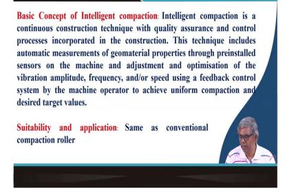
And basic concept of intelligent compaction already I have mentioned but once again I will organize way let me read once an intelligent compaction is a continuous construction technique with quality assurance and control process incorporated in the construction.
