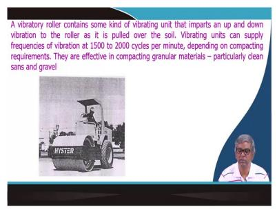
And then this is actually vibratory roller. I have already mentioned perhaps the sandy type of soil, granular soil. It is good regular soil actually when you will give some vibration then actually the smaller particles can enter easily the larger particle and more compact state we can be achieved.
