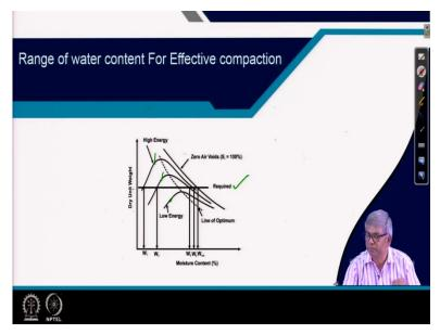
So, let me come to this slide, through this slide actually, as we have mentioned that there is a particular moisture content is very important for compaction particularly this by conventional shallow densification method and also, I have mentioned that, that if we use the same soil different energy level again the moisture requirement and maximum dry density achieved also will change.
