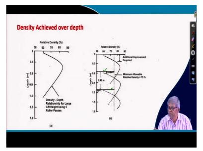
You can see here that when you compact by roller or by any means, on the surface, how density varies over depth. You can see here that it will not be densified at the surface. Maximum density will never be on the surface. You can see close to the surface density will be comparatively less and little deeper it will be maximum. And again, if you go further deeper the it will be density will be reduced.
