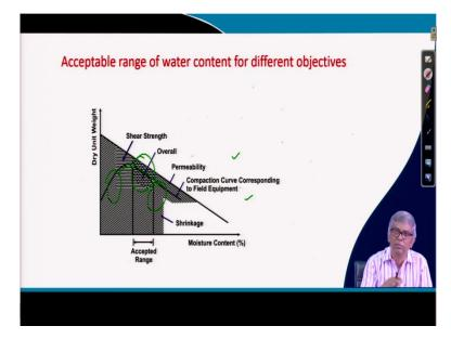
And here actually you can see that the total compaction curve and this is supposing a total compaction curve this one is that total compaction curve and then in these actually you cannot in the field particularly cannot compact at the optimum moisture content. If the if you can compact optimum moisture content then you will get maximum density obviously, but you cannot do that.
