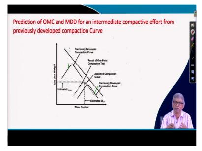
Now, sometime prediction of OMC MDD for an intermediate compactive effort from previously developed compaction capsules from the title I just read suppose, I have one compaction curve this, another compaction curve is these, but in the field and it has a definite amount of energy this is also definitely an ideal amount of energy and this has a zero air void lines and, in the field, I got some energy which is not same as either of these are these may be intermediate.
