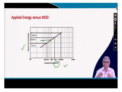
And here another thing is that I have shown that that when you increase the energy level that we apply more energy, then we get higher optimum higher maximum dry density. So, finally, if I do several tests several tests on the same soil on different energy level and finally, if you see that maximum dry density, it follows a particular pattern and that pattern is what actually?
