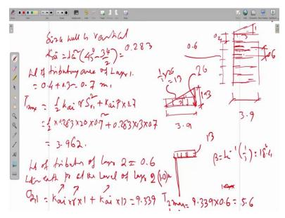
And here actually, so let me draw the wall first. There may be wall is something like this, some, 1, 2, 3, 4, 5, 6. So, these are the reinforcement. And this distance is 0.4, and these are all, 0.6 each, and this is actually 3.9. And this angle is 1 vertical, 3 horizontal, that means that beta is actually tan inverse 1 by 3, it gives you 18.4°.
