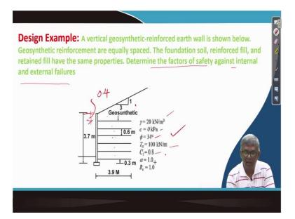
So let us come to the problem first. So, the problem is like this. A vertical geosynthetic reinforced earth wall is shown below. This is the one, is shown. What it is actually? The wall height is 3.7meter. And reinforcement initial, this is a trial design, suppose, and we have to check the factors of safety against internal and external. So, there are actually, 3.9meter long reinforcement is provided.
