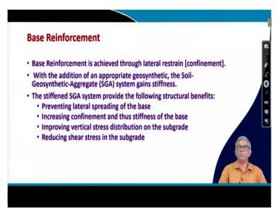
Here actually basically enforcement means what; that the below the bass actually that if the soil is not good enough, then we can use geosynthetics and this geosynthetics helps to improve the
