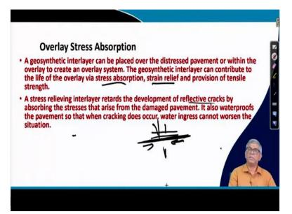
Next one, actually overlay stress absorption that is actually when if you apply stress if there is some mechanism to absorb, then sometime that cracking and other things will be avoided. So, it geosynthetic interlayer can be placed over the distressed pavement or within the overlay to create an overlay system.
