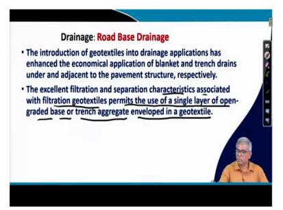
And drainage that is road base drainage, road-based drainage that is actually the interaction of geotextile into drainage application has enhanced the economical application of the blanket and trench drains, there are before actually blanket drain, trench drain is used. Now, because of these geosynthetics this can be more economically and quicker can be installed and that is actually under adjacent to the pavement.
