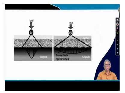
That mechanism is shown through this figure actually, you can see that before without reinforcement if this is the layer, this is top layer with sub base and subgrade, a base course and this is base course and this is a subgrade and this is suppose surface and the surface wheel is applied this figure already I have shown once, once again because it is relevant.
