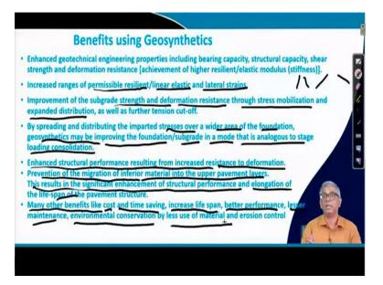
Finally, what if I use this geosynthetics in the different application what are the benefits. There are listed; enhanced geotechnical engineering properties including bearing capacity we have shown different example, because it is widening the stress. That means more load can take.
