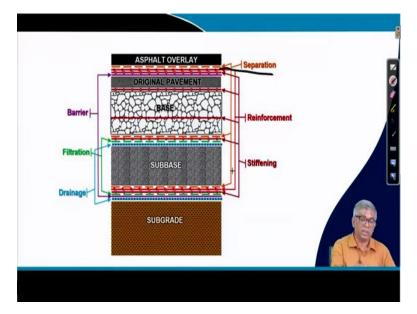
And you can see here in this figure actually use of reinforcement for various function, everything is given. But let us see only reinforcement. Reinforcement is here actually this is the reinforcement. And also, sometimes reinforcement is here also between this layer between these two layers, between this layer and this layer, there is enforcement is there.
