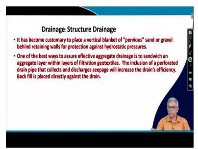
And then that one more let us see that drainage in structure drainage that means you know that when there is a retaining wall and we generally have backfilled and we know that free reading backfield to be used and in addition to that, behind the wall, there should be some drainage layer that water can drain easily instead of accumulating there. So, those are the application actually.
