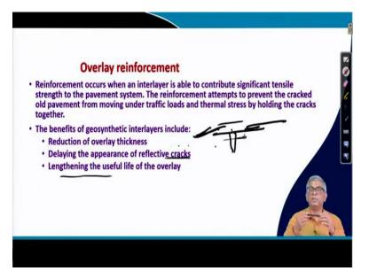
Next one overly reinforcement; overlay when it will be reinforcement occur when an interlayer is able to contribute significant standards tensile strength. Sometimes geosynthetics use in for different purposes like drainage or like separation, those purposes are there, but in addition to that, if it provides sufficient tensile strength, then that is called reinforcement actually.
