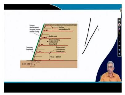
And you can see that whatever figure I have drawn that roughly it is similar you can see this reinforcement wrapped around, the reinforcement wrapped around like that quite steep flow we could make an whereas if I do not use this enforcement, the slope would have been like this. This is actually something like this.
