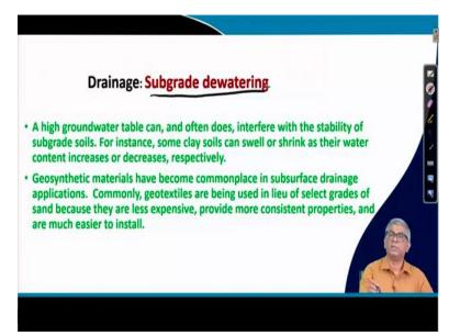
And next is whatever we have discussed that is regarding the road and pavement. Now for the geosynthetics can be used for drainage and drainage in subgrade dewatering, drainage, high groundwater whatever is there and that groundwater table that water when come in contact with some of the soil type which will come in contact with water either soil or when drying it sink and that actually creates problem.
