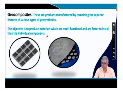
And next one is, you can see geocomposites, sometime that geogrid and it will be covered with some geotextile and it will solve some purpose, it will give some strength in addition to that you will provide as a drainage barrier, so that is what this is mentioned that these are products manufactured by combining the superior features of various types of geosynthetics.
