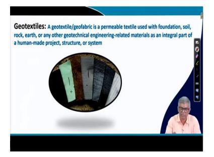
Next one is geotextiles. And this geotextile again from the name itself it is quite obvious textile means is like cloth and so, geotextile or geo fabric it is also known as geofabric is a permeable textile used with foundation, soil, rock, art or any other geotechnical engineering, related engineering related materials as an integral part of the human made project, structure or system.
