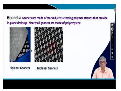
Next, will be geonets, and you can see from the name itself again it is quite obvious it will like net, geonets are made of stacked, cris-crossing polymers strands that provide in plane drainage actually can see it provides drainage and also there will be, this there are biplanar geonets, there are triplanar geonets and how it looks that it is shown here, it is shown here.
