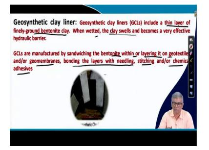
Next one, you can see geosynthetic clay liner. This is again a typical material which is also a combination of a number of things and it will be sometime clay liners, after, when we dump the waste and they are actually we give a clay liner to prevent, leach it, come out from that source and mixed with other groundwater or soil.
