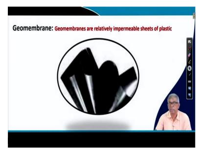
Next one is geomembrane and this membrane from the name itself is quite clear geomembranes are relatively impermeable sheets of plastics. So, when there is some permanent separation is required you do not want to permit something to move, pass through then this type of membranes are used.
