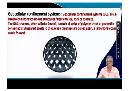
And geocellular confinement system here actually the first I can show in your picture itself, here actually you can see that geosynthetics is manufactured I such way, if you pull them then this type of opening will form, this type of opening form. This opening actually can be filled up with some soil or sand, good sand and then it will be cover, thin cover if you give then this layer will have a better effect than any other material, normal material.
