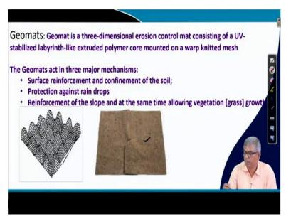
Next one, you can see geomats. Geomat is a three dimensional again erosion control mat consisting of a UV stabilized Labyrinth like extruded polymer core mounted on a wrap knitted mesh, we can see here from the figure at the bottom that this one, this can be wrapped and over that there is a, there is another cover, this together is name as geomet.
