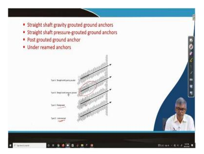
And there are, again anchor can be of different types, there are four types, type A, type B, type C, type D, straight shaft gravity grouted ground anchors. This is the one straight shaft gravity grouted and straight shaft pressure grouted, this is the one, then post grouted, this is the one and this is the under reamed. The different ways construction can be done so most common actually this one.
