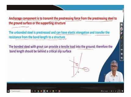
And then the anchor is component is to transmit the pre stressing force from the pre stressing steel to the ground surface. This is anchorage component; the function of the anchorage component is to transmit pre stressing force from the pre stressing steel to ground and the un bonded steel is pre stressed and can have elastic elongation and transfer the resistance from the bond length to the structure.
