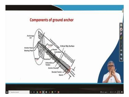
As I have told you that I will try to show you the more detail about this, you can see in this here that anchor is set, an anchor head is this one and then bearing plate is there and then you can see that this is actually bonded part, this is the bonded part, you can see anchor bond length, tendon bond length is mentioned, this is a bonded part and this is the un bonded part and this is the pillar surface.
