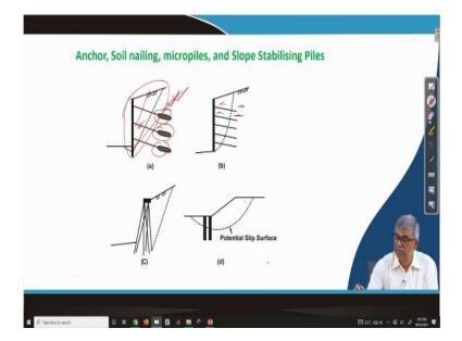
let us take the first slide that anchor, in the anchor before going to the anchor, let us show that similar things, different things which I will use, you can see here this is one, this is called soil anchor because you can see this is the active zone the soil will move along with wall and this is a resisting zone. Here main resistance will come from here, this is anchored they are sufficiently strong, you have to make strong so this anchor actually will be helping to stable this entire mass.
