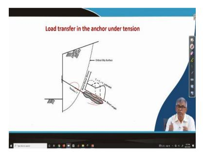
And load transfer in the anchor under tension. You can see here this is the one, this is the facing and this is the tendon and this is the anchor point. This entire thing will be in tension, this portion and under these what will be the load transfer mechanism in this zone, actually how it will be you can see here that when did if tension can vary because of many reason.
