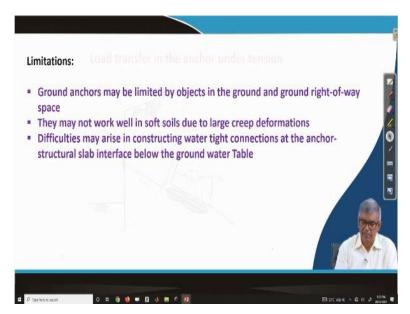
Limitations will be ground anchors may be limited by objects in the ground and ground right of way space and they may not work well in soft soil, that is obvious due to large creep deformation already mentioned that if there is a highly plastic soil organic soil because of this creep you need to take clear, but generally it should not be used, until and unless is very essential and if it is very essential to us then this can be used with a lot of care.
