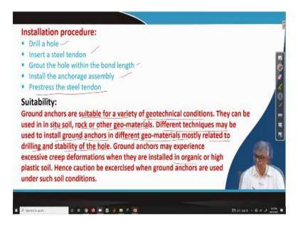
And installation procedure, you can see that first of all you had to make a drill hole and then installed a steel tendon, then grout the hole with the bond length, whatever that much portion to bonded, install the anchorage assembly and then pre stress the steel tendon, that is the steps in the construction.
