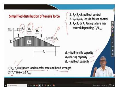
Again, then some simplified distribution of the tensile force. You can see though we have shown in the previous lecture module, that how the distribution of the other stress happens in the rod, we have seen that at the face, at the face there will be some value and then it will be increasing and then it will be decreasing and becoming zero. But here is then it will be curve continuously.
