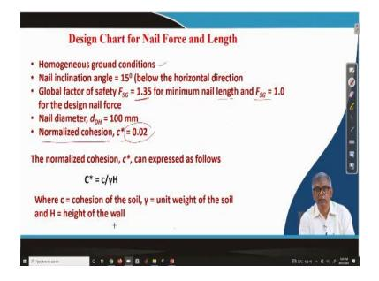
Next one is the design chart for nail force and length as all of our basic information is given based on that numerically they are analyzed and then there are some charts are given which can be utilized for the design purpose and what are those important assumptions are made in that chart preparation, homogeneous ground condition. So, ground behind the where nailing will be done, it has to be homogeneous, it may not be reality, but assumption is.
