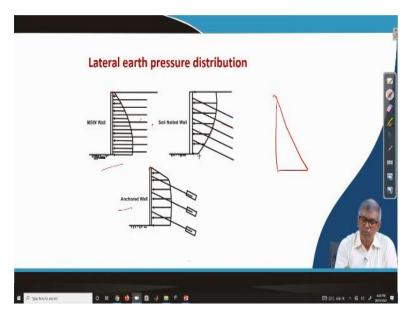
Let us take that one by one and you can see here, let us take your first slide here when ever with design wall, we have seen that in the soil mechanics or foundation engineering that we need to calculate that pressure, earth pressure and earth pressure when you do in the retaining wall, regular retaining wall generally we know that retaining wall earth pressure will be like that triangular.
