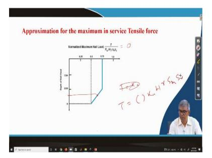
Then this is as we have mentioned that diagram, earth pressure diagram, so normalized maximum nail load and what about different height that is given diagram here and this will be up to two third H it will be constant and from two third H to H it will become reduced to a value 0.75 to 0.5 so this slope can be automatically obtained. So this is a guideline to depth of nail head to normalize maximum nail load, so that this is the diagram is given, can be utilized.
