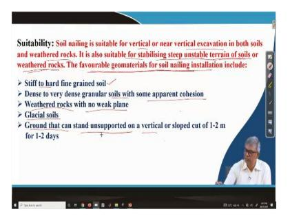
let me go to the next slide, suppose for everything whenever we have discussed that any method first of all whether it is suitable or not because of that you have to check suitability and where it will be suitable that we have to check and suitability of soil nailing, soil nailing is suitable for vertical or near vertical excavation, which I have shown in the beginning and vertical or near vertical excavation and both soils and weathered rocks, soil, rock both it can be like.
