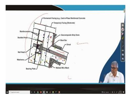
Let me go to the next slide, you can see that as I have told you that circle mark is enlarged here and you can see here detail and you can see here this is the main nail and then if it is a grouted then if we made hole and then nail is provided then this grouted portion that is to hold the soil within the soil mass that entire grout rod together, so this portion is grouted and this is the rod and this side is earth.
