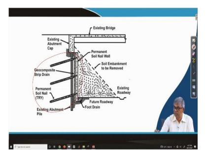
That here original abutment was this one and this was the pile foundation suppose and there may be some restoration is needed in that case we can have soil nailing in front of that like this, soil nailing in front of this soil nail wall can be made and this soil embankment to be removed, this if you want to remove then permanent soil, so originally this was the abutment and this was the soil position.
