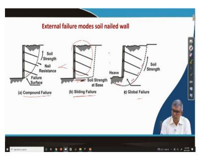
The external failure mode of soil nails wall and you can see again here number of them. Compound failure, you can see here that entire compound failure means it will be the soil will fail or if the nail will fail and here like this, so this is a compound failure and then soil, that will be sliding failure, there may be, this portion soil nail is quite tensile strain, quite bond strength between the soil and grout nail and between the grout and nail all those things are good.
