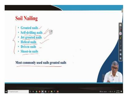
Then let me go to the next slide to show you some more information you can see now that the soil nailing as I have mentioned that it can be directly pushed or it can be the different ways it can be constructed, so what are the different ways it can be done, there will be grouted nails that means we can make a hole and with grout and the nail can be input, the grouted self drilling nails we can drill and then it can while drilling it will go inside that is self draining nails.
