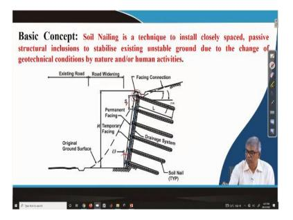
Let me take the first slide that is the basic concept as I have told you can see that it is a technique to install closely spaced passive structural inclusion to stabilize existing unstable ground due to the change of geotechnical condition by natural and or human activities. You can see whatever the because of the manmade or human or natural activity, natural or human activities and I will just give you the example of human activities first.
