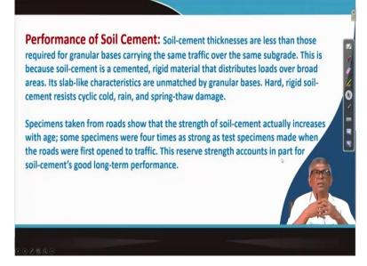
Let us go to the next one, the performance of the soil cement. The soil cement thickness is less than those required for granular base is carrying the same traffic. Suppose if you design for a particular volume of traffic and the base if you design for the normal granular material and cement treated material then obviously the thickness will be less when it is cementite.
