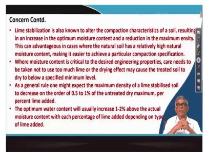
Then continue again further lime stabilization is also known to alter the compaction characteristic of soil, how? The resulting in an increase in the optimum moisture content that means when a lime treated soil, it increases the optimum moisture content and reduction in maximum density.
