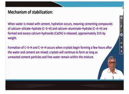
So, let me go to the next one and mechanism of stabilization, again similar to the lime how it works? Here also when water is mixed with cement then hydration occurs meaning cementing components of the calcium silicate hydrate that means reacting with water cement reacting with water that is calcium silicate hydrate that is (C-S-H) or calcium aluminate hydrate CAH are formed and excess calcium hydroxide is released approximately more, around 30% by weight.
