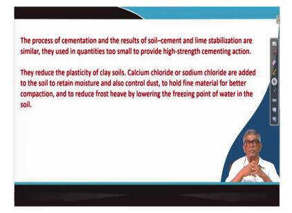
And this process of cementation and the results of soil cement and lime stabilization are similar. The process of cementation and the results of soil cement and soil stimulation are similar and they used in quantities too small to provide high strength cementing action. So, both cement and lime they are used in a smaller quantity and how small or how big that has to be investigated and then determined.
