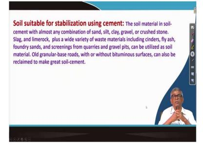
Let us see the next slides and suitable for stabilization using cement, the type of soil which we have mentioned in the lime, we have mentioned here also similar to that cement also can work with in many combinations of sand, silt, clay, gravel that means these are all different combination, gravel crushed stone, this can be used with cement to give improved properties.
