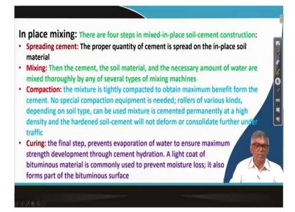
After mixing let us see the next step and then of course as I have mentioned that mixing can be done two different ways actually one is in the plant and it can be done in place mixing that means easy to mixing. There are four steps when you do in place mixing, the spreading of cement that means on the site, you have to spread the cement, quantity of cement is spread.
