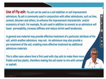
Then let me continue the last slide perhaps, the use of fly-ash. As I have mentioned that sometime additives, so fly-ash can be used as a soil stabilizer or soil improvement mixture
