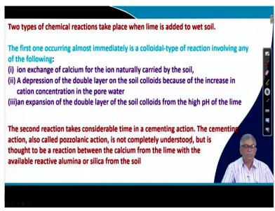
Let me go to the next slide, so two types of chemical reaction take place when lime is added to wet soil and first one occurring almost immediately that out of two, the first one almost immediately and is colloidal type reaction involving any of the following. There are three different types of things can happen during that, iron exchange of calcium for the iron naturally carried by the soil.
