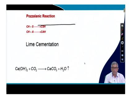
And as we have mentioned before that this is symbolically written actually calcium hydride and silicate CSH, this is standard form which we will use CH and aluminium. Actually, with lime and the silica present in soil or alumina present in soil, can react with that and then it will form a stable CSH or CAH and again another reaction happened with the carbon dioxide with this, the calcium carbonate form and water will form. So, this is also helps to stabilize the thing
