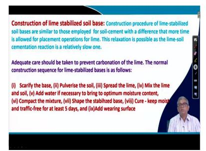
Construction of lime stabilized soil base and how we can do this? There are certain steps actually, the adequate care should be taken to prevent carbonation of the line. The normal construction sequence for lime stabilized bases will be a number of them there are 8 or 9 steps are there you can see, scarifying the base, that is scarifying the basement surface, first of all by using some you have to make it rough. And surface will be scrap and then you have to make it actually soil lamp form.
