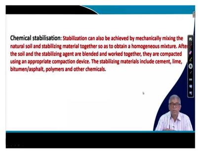
That is actually if I do that it is called mechanical stabilization. And similarly, we can think of chemical, when it is a chemical stabilization, it is achieved by mechanically mixing the natural soil and stabilizing material together so as to obtain a homogeneous mixture and after the soil and the stabilizing measurement are blended and work together, they are compacted using an appropriate compaction device.
