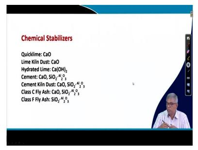
We will try to concentrate now on chemical stabilization. When you do chemical stabilization then actually some different kinds or different types of chemicals will be used and that is actually lime is one of the most important chemicals which is used in stabilizing soil.
