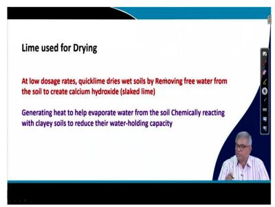
Let us take one by one, so lime used for drying, when you use it for drying, it will low doors will be used and quick lime dries wet soil. Actually, when the wet soil if you add like quick lime then it will help to dry the soil by removing free water from the soil to create calcium hydroxide. This is one and while doing this reaction it generates heats and that heat cycle to help to evaporate water from the soil chemically reacting with clay soils to reduce their water holding capacity.
