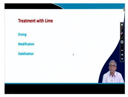
We will try to see now what are the way we can do this. Treatment with lime, now I will try to concentrate on use of lime in stabilizing the soil and you can see, we have mentioned that if the moisture is reduced from the soil, generally soil characteristics will be improved so drying by applying lime we can dry the soil and we can by applying lime we can modify the soil and by applying the lime we can stabilize the soil. So, these three different ways lime can be used for improving the soil.
