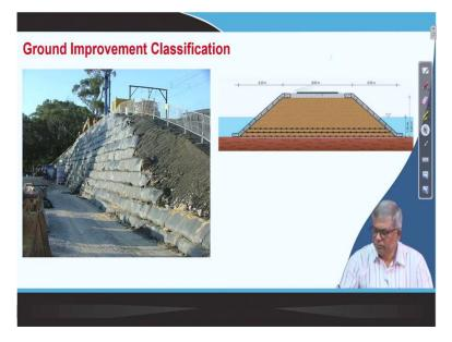
So, this is actually you can see here when it is a slope and when it is making embankment. So, these are the two examples are shown already here and which I have tried to sketch and you can see that these are the different level of reinforcement has provided different level and then this slope is provided. So, when you provided these, then automatically it will not be able to slide like this.
