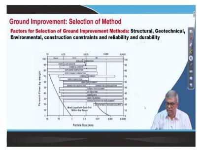
Next slide you can here, that when we have several factors actually the factors include structural factors then, what type of structure you will make? Geotechnical factors, environmental factors, construction constrain and reliability and durability. So, many factors will be there, all those things to be examined, and in addition to that, what you have to see, you have to see the soil and when you see the soil.
