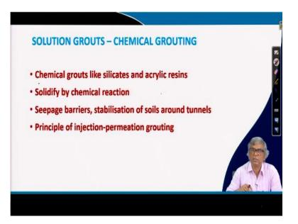
Then solution grouts, and here you can see solution grouts is a commercially available chemical grout, two or more materials are mixed, chemical grouts like silicates and acrylic resins. They are actually available, we will discuss later on also and it solidify by chemically reactions with soil sometime and they are used as seepage barriers, stabilization of soil around tunnels and most of the time these solution grouts out of there are several modes, generally permeation modes are used.
