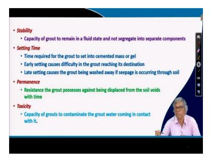
The stability, stability means exactly what? Stability means capacity of grout to remain in a fluid state and not segregate into separate components. That is stability, you have to prepare the grout material in such way it will be in a particular, remain in a fluid state and like if I make a solution and after sometime the solid part settling and liquid part coming up that will not be a good grout material, when it will remain in suspension that is actually the stability of the grout material.
