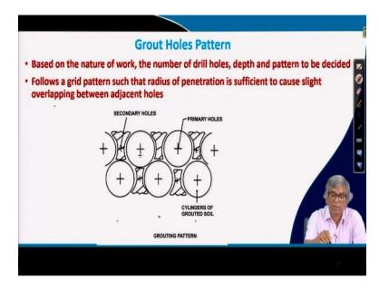
The grout holds pattern you can see here like in deep dynamic compaction or plate, repeated plate, impact load, then whatever other methods of grouting there actually we have shown that pattern and different, even preloading also if you make the different patterns, here also we can have similar different types of patterns.
