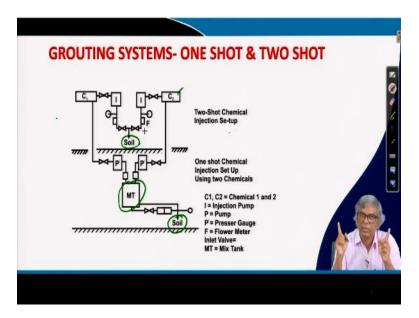
Now when you make the grout, there are two ways the grouting can be there, can be made. One is called one shot method and another is called two shot method. The primary difference between these two is, one shot means it will be mixed beforehand and injected to the soil together once, that is one shot and two shots means it will be injected once a, first one solution and after sometime again we inject the second one, that is two shots, twice we have to inject.
