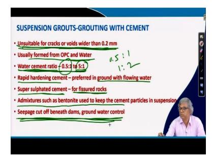
And let us further discuss about their characteristics and about suspension grouts. You can see suspension grouts and grouting with cement generally, suspension grout mostly with cement and sometime with clay also and if it is then it is where we can use or where we cannot use that some sort of discussion.
