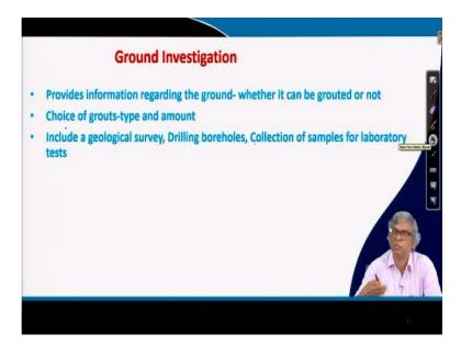
Next is ground investigation, under these so ground investigation, so here it provides information regarding the ground whether it can be grouted or not. That means first of all if the material is a typical one and where grouting is done, groutability that whatever we have mentioned that define all those calculations to be done after ground investigation.
