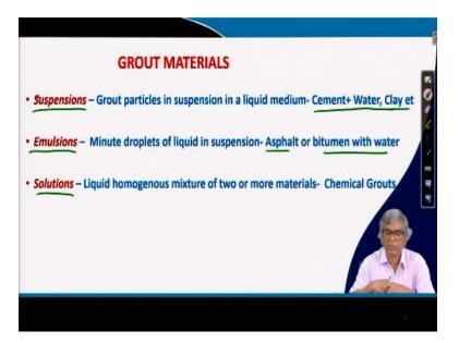
And then groutability you have done this, now grout material then again, we have understood that there is a suspension in the liquid form to be injected and then what are the different forms of grouts available and we can see here, there are three different, one is suspension grout, other emulsions grouts, another is solution grounds.
