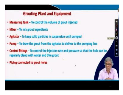
The grouting plant and equipment, so it will have a several components, the measuring tank to control the volume of grout need to be injected, so it has definite amount should be there. Mixer, to mix grout ingredients, then agitator, to keep solid particles in suspension until pump, you might have seen also ready-mix concrete when it is transported from the factory to the site there will be drum always will be rotated because to keep the agitating.
