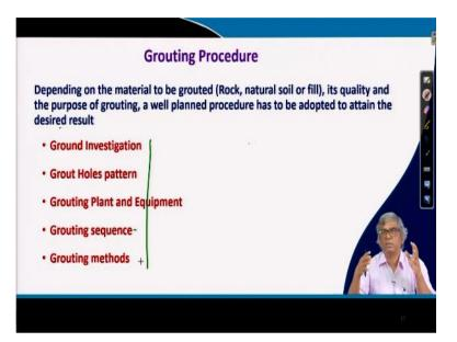
And grouting procedure. At a particular site suppose a grouting is chosen as a one of the ground improvement techniques, then how will you proceed, just will not go to the site and inject the chemical, it is not, you have to have certain procedure depending on the material to be grouted, whether it is rock, whether it is a natural soil or it is a fill its quality and the purpose of grouting a well-planned, procedure has to be adopted to attain the desired results.
