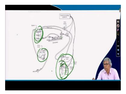
These are actually plant, there are various components and I will show the overall sketch of this plant, you can see here number of things will be there, this is the, you can see here finally grouting will be done here and it is grout mixer and you can see this is agitator, after mixing we can put it here and it will be if it is not pumped then it will be kept on agitating.
