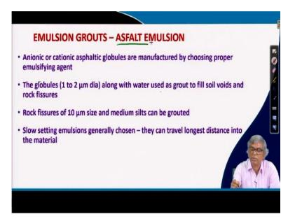
Then emulsion grout, anionic or cationic asphaltic globules are manufactured by choosing proper emulsifying agent. That is the manufacturing process, the globules 1 to 2 micrometer diameter, that is the size, along with water used as grout to fill soil voids and rock fissures. They are used actually to fill the soil voids and the rock fissures and size is 1 to 2 micrometer and they are droplets in the water. Rock fissures of 10 micrometer size and medium silts can be grouted also.
