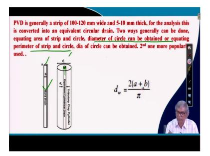
And let me go to the, so PVD, what is PVD actually? PVD is actually, is a strip and it is generally 100millimeter to 120millimeter wider, wide and your and about 5 to 10millimeter thickness. And for the analysis purpose generally, if you have. So, if you have this one, this is the strip suppose and it will have dimension a, b and it will have thickness. So, a is the thickness, b is the width.
