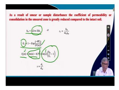
you can see now, here you can see kh is actually or  $k_r$ , it is 2 to 3 times of ks. The smeared zone, the k value will be reduced. And then Ur can be calculated, again same equation. But  $F_{sn}$  when it is a smear, that k is actually  $F_{sn}$ . And that can be calculated when smearing effect is consider, the equation, our equation was previously up to this but additionally, this portion to be added. Ln s multiplied by  $k_h$  by  $k_s$  minus 1.
