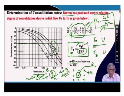
let me come to this one. This is the one we have, we have shown before. This is the equation you can see; the time and you use the pore pressure. And you can see that the other thing  $C_v$  is there, coefficient of consolidation, z is there, the direction and r is the radial direction.  $C_h$  is the coefficient of pressure horizontal direction. And  $C_v$  is the coefficient of consolidation in vertical direction.
