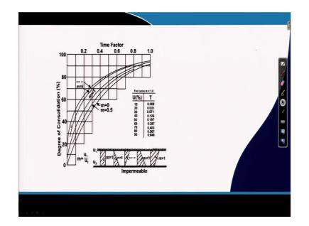
So, so, you can see the, from the theory we have seen delta c equal to what? Mv multiplied by delta p multiplied by H. So, these values are known. So, mv value actually is given 2.5 multiplied by 10 to the minus 4. So, divide by this one, multiplied by delta p is 100 kilonewton per meter square. And your thickness of the layer is 9.2 since it is one direction.
