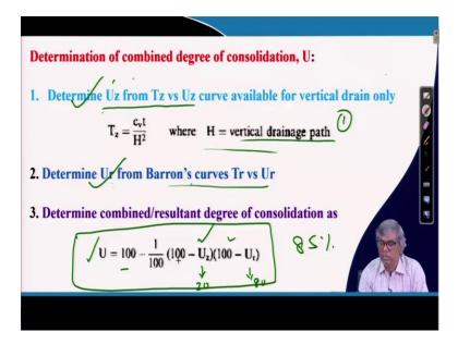
You can see here, for finding out the consolidation problem, in with radial drainage, at any time how to find out the Tv of consolidation you can see here, that step one that determine  $U_z$  from  $T_z$ versus  $U_z$ . Determine  $U_z$  versus  $T_z$ . So, how much a settlement actually required or how much, how much settlement, total settlement will be there, how much do we achieve? From there you will be getting U, and from U, and  $U_z$  versus  $T_z$  curve you can find out  $T_z$ .
