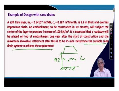
You can see that, this is the one. A soft clay layer which is having mv equal to 2.5 into 10 to the power minus 4meter square per kilonewton and  $C_v$  equal to 0.87meter square per month, this is actually two soil parameters are given. And that is clearly, its thickness is 9.2 meter thick. And overlies impervious shale, impervious shale. That means one direction drain.
