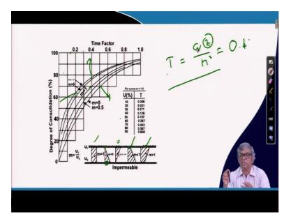
And here actually you can see, that this is the solution for radial drainage. And this is the solution for vertical drainage. This is, I have not, this one I have not shown because this is done in soil mechanics. Only thing actually here actually there are too many curves, but all may not be useful. You can see here, that when there is a load is applied, pore pressure within the soil can be assumed uniform.
