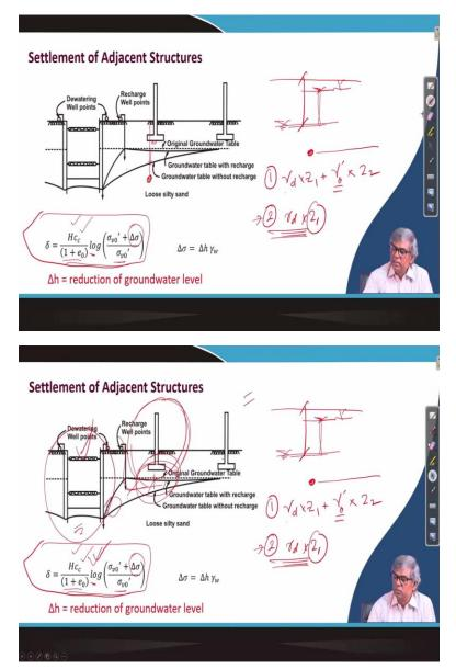
Then another thing is sometime that I have also mentioned before that recharge well point our topic main topic here actually in this module is the dewatering that means, by pumping water you had to lower the water table from a particular level to particular level for the ease of construction. So, here suppose we this is the construction point and you have to lower the water table because of that suppose you have done well point some arrangement you have done and based on that water table.
