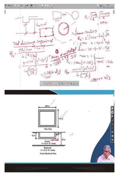
Suppose let me take. So, from here actually when there is a rectangular area, rectangular area of suppose this 170 by 220 then we can imagine this as an equivalent circular area, if I imagine that, then I can find out that equal and radius are not will be equal to under root L multiplied by B divided by pi. That means, it will be under root 220 multiplied by 170 divided by pi so this will be equal to 109meter.
