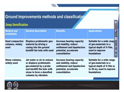
Next one is about again Deep Densification, it is continuation. There are different ways we can do, one is by Weight falling up weight and then we can do by Vibration compaction there are another a few more methods out there, that is Sand Compaction columns. It means we can buy a Displace problematic geo-material by driving a casing into the ground backfill the hole with sand.
