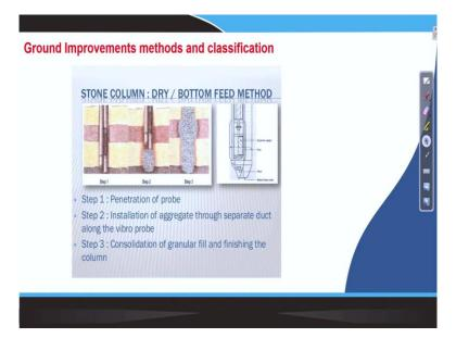
The next method so this is actually typically shown a diagram of the stone column actually you can see that this is the one first shown the step one that Penetration of probe then step two, the Installation of aggregate through separate duct actually then along the vibro probe and then step three Consolidation of granular field and pre leasing the column. So, these three steps actually, sometimes it is done that is Dry Bottom Feed method actually. Stone column this is called Bottom Feed method.
