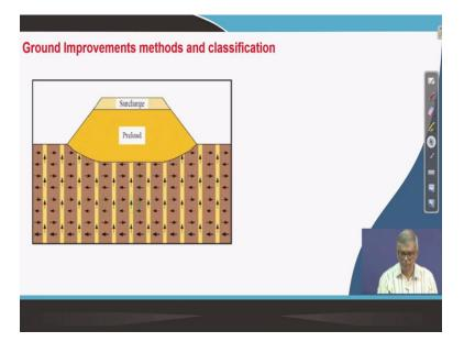
And this is the way you can see here in this diagram you observe the soil, this is the soft soil it is to be consolidated. And if you apply this much amount of surcharge, then over the time, actually soil will undergo this then you can see that it was the level which was initially here and then you can see, initially the level was here and because of the surcharge it has come here.
