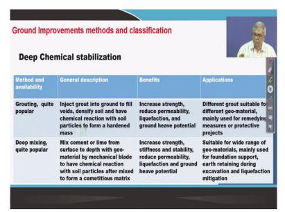
Then next one is the Deep Chemical Stabilization you can see here the deep. Deep means quite deep, actually different methods again use the deep chemical compaction stabilization here actually grouting is there and then there is deep mixing, two methods are there when it is the grouting it is quite common popular already I have mentioned and how it works actually inject grout into ground to fill voids.
