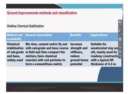
Next one is a Shallow Chemical Stabilization again, Shallow Chemical Stabilization in the surface soil like the embankment to be made and the soil we are using maybe some lime or something can be added and mixed later then roller then sometime we can keep and with some reaction soil will be improved to that is why. So a chemical stabilization of sub-grade and base widely used.
