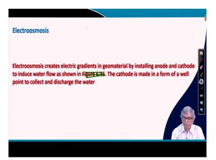
Next one, for example, Electroosmosis. As I have told you, so far, the soil should be permeability should be high. So that if you discharge water and lower in a particular zone, then from the water from the side will be moved to that zone and again it will be pumped out. Ultimately influence area will be so if I pump from here the influence it will be in initially at this point, but surely, if you continuously pump water then slowly the influence area will be increased.
