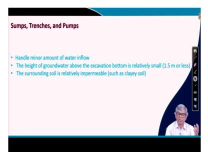
And you can see sump, trench and pumps. In this as I have already mentioned handle minor amount of water inflow. Not a large quantity of water because it is by gravity flow only. And the height of groundwater above the excavation bottom is relatively small. Height of groundwater above the excavation bottom is relatively small than that can be managed and it is actually maybe in the range of 1.5 meter.
