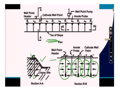
You can see here this is the typical electroosmosis, this is suppose the plan view and you can see anode and cathode this is anode, cathode anode cathode like this and if I take a section here and you can elevation if you see, you can see this is the elevation you can see here, this is the cathode point and then water will be moving towards this one and this will be treated as well point system and through the pump water pump water can be taken away and then slowly water level will be lowered.
