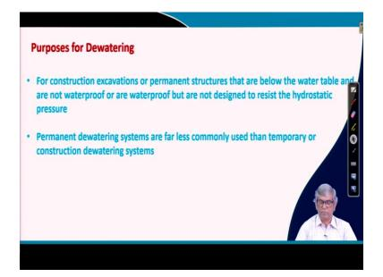
It is purpose for dewatering it is already I have mentioned that most of the for-construction excavation that means, when you want to build a building or anything else you need to have foundations particularly if the shallow foundation, then you need to excavate and if it is deep foundation, obviously, you generally a pile foundation can be done without excavation, but sometimes is required to excavate up to some depth.
