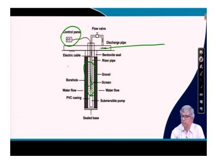
Let me come to the next point and this is the, this is the figure for corresponding to this method and you can see here this is the pump as I have told that you have to make the hole and it will bottom will be sealed with particular way, that water should be entered only collected from this level only, and this is the one actually this is the pump and this is with PVC casing and here will be screen this is the screen material.
