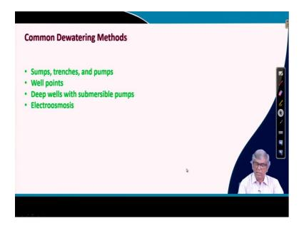
Let me see this. Then there are different ways that dewatering can be done. Dewatering means actually what the original ground level is somewhere and to facilitate the construction or, or other activity, you have to lower the groundwater table, how you can lower the groundwater table? You can pump water, and generally, water table means actually maintaining parallel through ground surface and will be horizontally maybe infinitely both sides will be extended.
