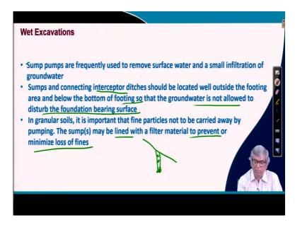
That this is actually about the precautions actually when you do by these some pump frequently used to remove surface water and small infiltration of groundwater. What there will be rain actually to infiltration and that infiltration of joining to ground or before that it can be collected to trench and through that it can be pumped out and then, then that is the that water table should not go goes up that can be maintained.
