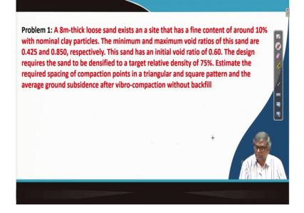
You can see that this problem is described like this, 8meter thick loose sand exist at a site that has a fine content of around 10 percent with nominal clay particles. If there is a too much of clay particles, it will not work. And it has a silty loose sand that is also good for vibro-compaction. The minimum and maximum void ratio of the sand are 0.425 and 0.850 respectively.
