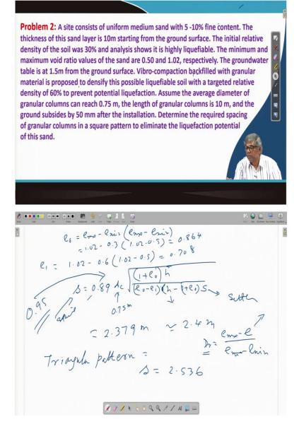
This problem is you can see now, a site consists of uniform medium sand with 5 to 10 percent fine content. The thickness of the sand layer is 10 meters starting from the ground surface. The initial relative density of the soil was 30 percent and analysis show it is highly liquefiable. The minimum and maximum void ratio was minimum and minimum void ratio or max to 0.5 and 1.02.
