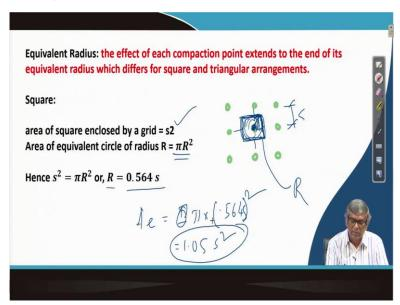
Equivalent radius. You know that a square pattern, suppose this one and this one, this is a square pattern. And then what I can find that area of influence can be of this, of this, and this. This distance will be half of spacing, again this distance again half of spacing, this distance
