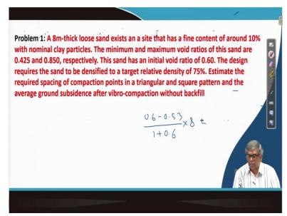
Here you can see the sand has initial void ratio 0.6. So, if you do that that means one 0.6 minus 0.53 divided by 1 plus 0.6 multiplied by 8meter. That become your deformation. So, it will be 0.6 minus 0.53, 0.6 minus 0.53 divided by 1.6 multiplied by 8. It will point 35.
