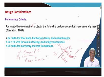
That design consideration in the Vibro-Compaction, the performance criteria first of all, and now, for most Vibro-Compaction project, there are a few things, most important thing to be considered the relative density and relative density for all projects, it may not be same relative density when it is slab or flat bottom tanks and embankments.
