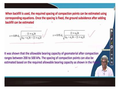
And this is the one when backfill is used the corresponding equation is when subsistence is there, already just the initial lecture I have discussed this equation we used for square pattern and this is the equation to be used in a triangular pattern. Also, it is shown that after compaction that the range of bearing capacity fall between 200 to 500. Sometime using that also people can find out the spacing that is given in the next slide.
