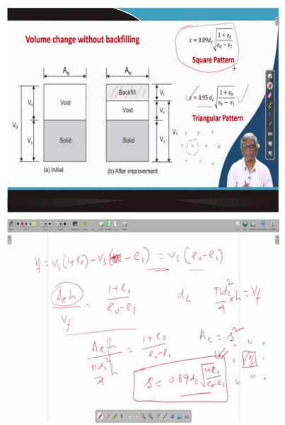
This is actually when you do with backfilling then this is the one and then you can see that initial these much voids. Now, it is backfilled, then it will be same level will be maintained. How that can be, from this how you can find out a spacing that can be seen. And you can see that  $V_f$  equal to nothing but Vs multiplied by 1 plus e naught minus Vs into 1 plus 1 minus e1. This one if I do and then it is nothing but Vs multiplied by e naught minus e1.
