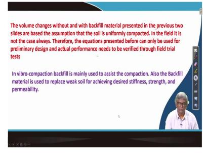
So, next, the volume change without and with backfill material presented whatever just you have discussed how to find out the spacing and all. And this is while deriving these it is assumed that the soil is uniformly compacted, but in practice is hardly it happens. This equation and because of that equation can be used for your preliminary assessment or preliminary design, but final design can be obtained based on our final decision can be taken based on trial test in the field.
