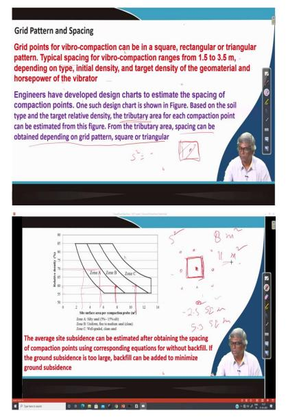
So, grid pattern and spacing, you can grid pattern in of course in Vibro-Compaction in general there are many, many ground improvement techniques there are you have to prove and you have to make a hole and then you have to use some material that is there are different patterns or you generally square and triangular pattern is very, very popular, but here Vibro-Compaction sometime rectangular pattern also can be used.
