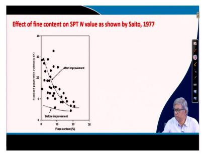
You can see this figure, that here actually standard penetration value and this side is fine content and you can see 10 percent, 20 percent and you can see here that before improvement, the standard penetration value with fine content, this is the line approximately so and after vibro-compaction, the fine content with your SPT value we can see that these are the value and the average line is drawn here, this is after improvement.
