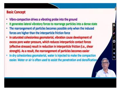
The basic concept in it that is, there is a probe that will be driven into the ground. And then, it will generate lateral vibratory forces to rearrange particle into a dense state. This rearrangement of particles become possible only when the induced forces are higher than the interparticle forces.
