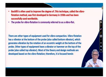
And, sometimes backfill so when this operation will be done, then automatically this will be subsidence and so that to make our soil to be densified at a depth. Sometime, we can backfill it and then backfilling will go that place is vacuum created and that place again, it will be further compacted and further more compact soil can be prepared. Without backfill also it is possible.
