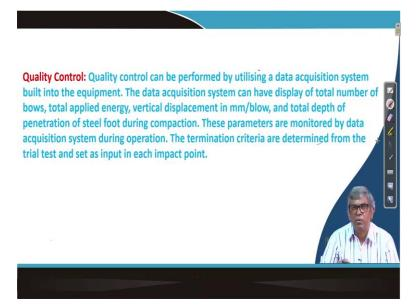
Next slide will be quality of course not much quality under it is there. A quality control can be performed by utilizing a data acquisition system in this particularly in rapid impact compaction data acquisition system can be used. Which is the built into the equipment. And the data acquisition system can have display of total number of blows, total applied energy, vertical displacement in millimeter per blow.
