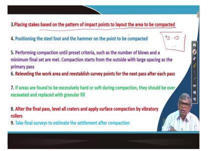
And next one will be your placing the stakes based on the pattern of impact to layout the area has to be compacted. That means your area is there. Then you had to mark actually where actually that the impact by rapid impact compaction that foot plate will be placed. That has to be marked properly. You have to go to that place and then required number of blows will give there and then move to the next. So, that is third step.
