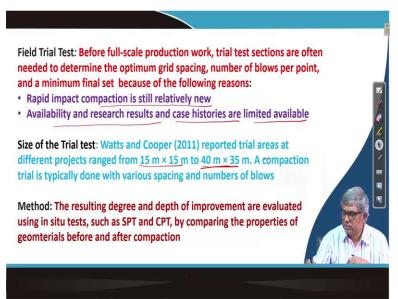
And next is actually you have to so these are the design that means design means what I have decided the depth of improvement and then I have decided hammer weight, I decided drop of hammer height, height of hammer drop, then I have the decided the size of the plate footplate, I
