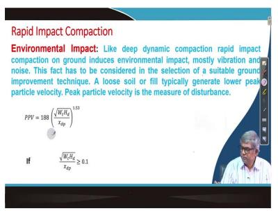
So, let me see in this one hour like in your deep dynamic compaction the rapid impact compaction also produces a vibration or health or environmental impact or environmental hazard. And these environmental hazards sometimes because of that we cannot select every any site these type of activities. So, you have to do some calculation and you have to see that you are not making any value which is exceeding some regulated values.
