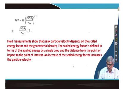
You can see here that this is the PPV equal to 36 and under root W2 Wt instead of Wt it can use  $W_h H_d$  divided by  $X_{dp}$  to the power 0.79. So, this equation can be used and if this value is this value is less than 0.1. So, now some as I was telling that some term the field measurement show that peak particle velocity depends on the scaled the energy factor. So, this is the one is called scaled energy factor, scaled energy factor means what is it, how it is defined?
