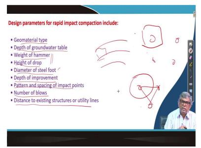
Next one is the design parameter for rapid impact compaction that you have to find a finalized already you have discussed certain point I have listed here. And we can see here the most important part is geometrical type the all material cannot be compacted by rapid impact compaction it is generally granular type of soil, silty sand, and all can we add some fill. So, that is what you have to see that is most important parameter for rapid impact compaction.
