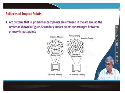
Then there is a pattern or the impact that is very important as it was in a deep dynamic compaction here also similar since it is an excavator is used which can be moved different direction and fixed in a particular location. So, there is an arc pattern there is a method is an arc pattern you can see this is the excavator and you can move either this direction or that direction and you can see if this is the so with this standing here it can give impact here, here like this.
