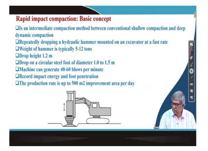
And you can see this that whatever I have said already that rapid impact compaction. This is the weight actually, it is and this is the plate it will be fixed in the, and this is by hydraulic arrangement. This one lifted up to this much height and again is allowed to fall here. That way it can be given within a short time a good number of blows can be applied here. So, this is the machine basically and this is some excavator actually can be attached to this one and by that this can be done.
