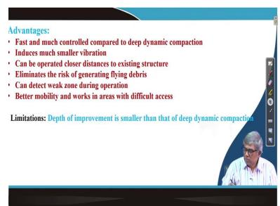
And some advantages that means so far whatever we have used, discussed that is shallow densification then deep dynamic densification with respect to that what is the advantage here? First and much controlled compaction to deep dynamic compared to deep dynamic compaction.
