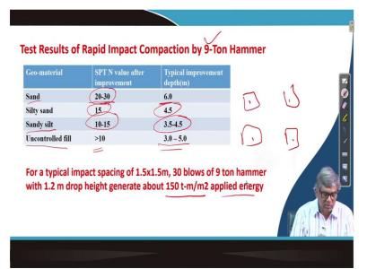
And see the results of rapid impact compaction by 9 ton, hammer a 9ton hammer is used and in that for different geo-material suppose if the sand is taken and SPTN value 9ton hammer then after compaction their typical improvement depth is 6meter. And in that case the SPT value can be after compaction can be up to in between 20 to 30. And if it is silty sand the SPT value can be achieved by deep dynamic compaction 15 and it can be improved up to depth of 4.5 meter by using 9ton hammer.
