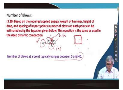
Now, number of blows here actually since ironing pass is not required. Whatever amount of energy required whatever I have shown in the table different type of soil and how what is the energy requirement. This energy is totally applied by the rapid impact compaction in no calculation though we may use at the end a roller that calculation is a small amount we cannot be separated. So, total required energy.
