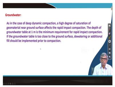
And next will be the groundwater and when there is a groundwater obviously like deep dynamic compaction will not be so easy. Here also it is so and actually the minimum requirement is groundwater should be below 1 meter depth. And if the water table comes above water 1 meter or within 1 meter in that case actually sometime you dewatering will be required or sometime additional filling can be used.
