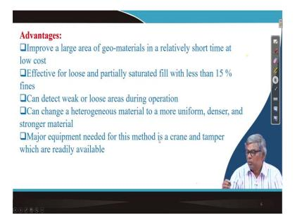
What are the advantages? You can see that when we have discussed about shallow densification with respect to these, what is the advantage of this method. It improves a large area of geo materials in a relatively short time at low cost that is the most important, very quickly it can be done. And first of all, its depth of improvement is quite high and very quickly and large area can be covered.
