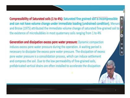
Compensability of saturated soil 1 to 4percent as I have mentioned, saturated fine grain soil is incompressible and cannot have volume change under immediate loading undrained condition. And so, Menard and Broise actually 1975 activated the immediate volume change of saturate fine grain soil to the existence of my micro bubbles in most quaternary soils ranging from and 1 to 4percent.
