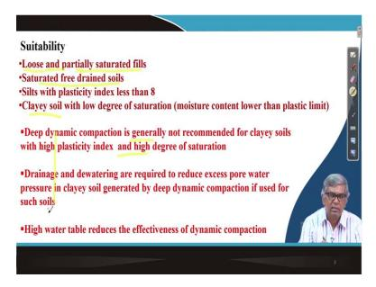
And you can see suitability; suitability means actually, you can see that where actually we can, we can use this deep dynamic compaction effectively. The most important is that loose sand and partially saturated fills, loose, loose and partially saturated fields and then saturated free drained soils. So, this is another important thing.
