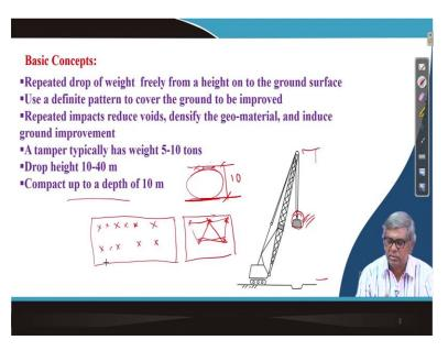
Let me take the first slide, that it is the basic concepts. As I have mentioned that, repeated drop of weight freely from a height onto the ground surface. You can see here that, you can see this is the weight and this is the ground and it is lifted this much height and then through this crane and then finally allowed to fall on this ground.
