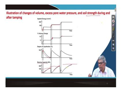
And this is actually illustration of changes of volume, excess pore water pressure, and soil strength during and after tamping. You can see here that different things are there when the applied load. Suppose 3 drops I have applied. So, one when applied load is there with time. This is the time within time load is applied actually, within this time load is applied, then this constant, so this much time we have waited, then second drop we have applied.
