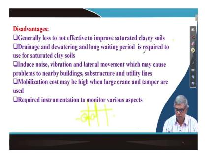
You can see number of disadvantages will be there, generally less to not effective to improve saturated clay soil. This is most important, saturated soil if you want to improve then we have to make some arrangements actually, otherwise just falling weight it will not help to improve the soil. Drainage and the watering and long waiting period are required to use for saturated clay soil.
