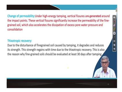
And next part is the change of permeability under high energy tamping, vertical fissures are generated around the impact points. These vertical fissures significantly increase the permeability of the fine grain soil, which also accelerate the dissipation of excess pore water pressure and consolidation. That means, when the weight falls the lot of fissures and cracks in form and through that cracks water also can seep through that will help to dissipation of pore pressure.
