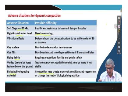
You can see here that the adverse situation for dynamic compaction where actually we cannot use dynamic compaction, deep dynamic compaction and if we use what are the difficulties. Actually, you can see that adverse situation is soft clays, where actually your Cu value that where under shear strength is less than 10, 30 that soil will be treated as soft soil.
