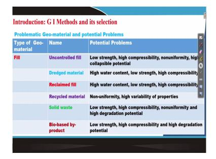
Next go to the Fill soil. Different again where soils at a particular site can be developed by filling material and different types of Fill can be used. One first type of Fill is Uncontrolled Fill, and it has some problems: It will have low strength, have high compressibility, has nonuniformity, high collapsible potential.
