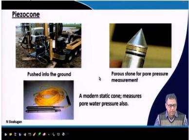
Now modern static cone test the pore pressure can also be measured. So, here we can also have cone resistance friction resistance we can measure as well as the same time we can measure the pore pressure also by using modern static cone penetration test all this piezocone which is called the piezocone.
