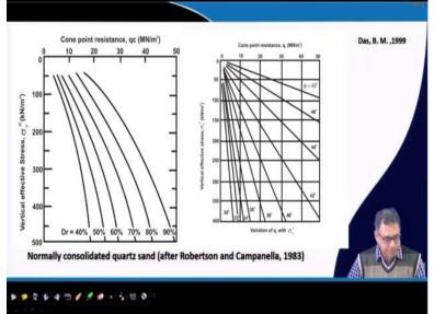
And we have different charts also by which also we can determine that soil relative density or the friction angle. So, this is what the sand if I know the cone resistance if I know the vertical effective stress or vertical overburden pressure, so, we know these values and the cone resistance then you will get the relative density of the soil and we will get the different friction angle of the soil also.
