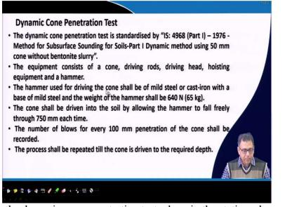
Now, next one is the dynamic cone penetration test where in the static code penetration test it is pushed into the soil, but here it is inserted into the soil by hammer blow which is similar to the SPT. So, here also the hammer blow, hammer weight is 65 kg and with a free fall of 750 millimeter and number of blows required for every 100 millimeter penetration is recorded. And these processes repeated up to the required depth.
