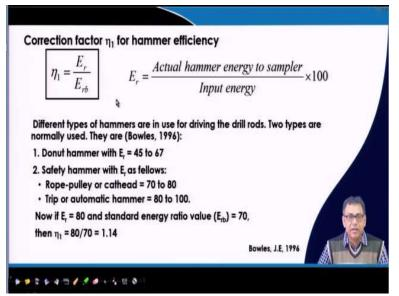
Now, what is hammer efficiency correction, this hammer efficiency correction is the ratio of  $E_r$  and  $E_{rb}$  what is  $E_r$ ?  $E_r$  means because we know that these are for standard penetration tests this is the hammer weight and this hammer height of fall is this much so, we know there is a standard energy that we are applying during the blows. So, that means we know that this is my height this is the weight. So, this will be the freefall so that means everything is standard.
