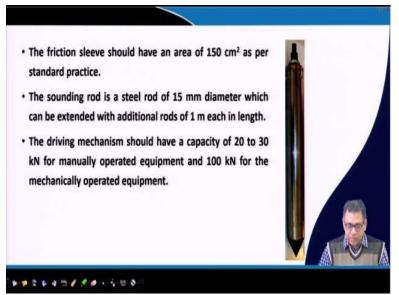
And these friction jacket friction sleeve or this sleeve outside area is 150 square centimeter. Now, sounding rod is a 50 millimeter diameter generally this length is 1 meter each, but we can extend the length of this or length of this cone by attaching additional rods of 1 millimeter each as I mentioned, so, this is the rod you can attach another one and then you can put you can go up to the required depth.
