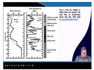
After doing the SPT and CPT static cone penetration tests finally we will get this type of data. So, this is the SPT blow count with depth S1 and S2 are 2 different boreholes and this is the SPT cone resistance only cone resistance along with depth for 2 different boreholes C1 and C2 and we can identify the soil also because by SPT we can bring the soil or the by the in borehole also we can identify soil. So, this is the soil type and this is the cone resistance and this is this the SPT value.
