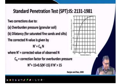
So, as per IS code that we have to apply the overburden pressure and the dilatancy correction. So, this overburden pressure correction is applicable for granular soil and the dilatancy correction applicable for saturated fine sand and the silt. So, in that sense if the soil is clay then no corrections are required. So, corrections are required for granular soil or silty soil. And I have discussed why this overburden pressure correction is required and dilatancy correction is required.
