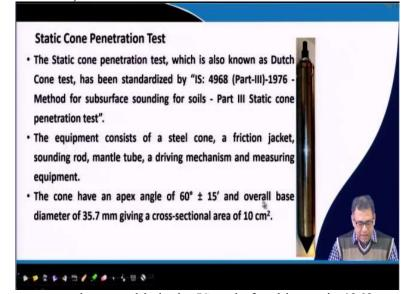
So, the static cone penetration test this is the IS code for this test is 4968 part 3, 1976. So, the equipment those are used here the steel cone then friction jacket sounding rod this is the sounding rod and driving mechanism and measuring equipments the angle this cone angle is 60 degrees plus minus 15 minutes and overall base diameter is 35.7 millimeter with a cross section of 10 centimeters square.
