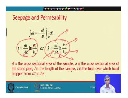
So, I have started initial time I have fixed zero and final I have time is t, suppose some 10 second or 1 day or 2 days, and h 1 and h 2 this is a two head, initial head is given 10 meter, final head given is 2 meter. So, this two to be observed, and then if I put this, then this one will be reduced to this form. And then finally, simplify this k become equal to al by At into ln, h 1 by h 2.
