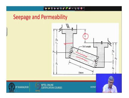
Now, let me go to next. So, this is the how to calculate the head that this figure is shown here. Suppose this is the soil mass, this is soil mass through which water taking place, flow is taking place. And if total head at this point, and total head at this point. If I lower this one lower this tank at this height equal to this, then there will be not any flow between this through this.
