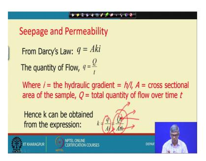
So, this is the application I will show, the equation I will show the next slide; that is you know that our equation is, k equal to your Aki, where A is the cross section area through which flow is taking place, that with Q, because V is equal to ki, and if I want to find out q, then I have multiply by A, and then this is the general formula and Q is equal to from the observation, this is a quantity over at time t I have taken.
