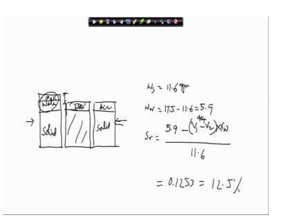
This is the one, we have the soil mass, and suppose initially this was solid, and this was water, and when water is removed in the mixer, then the volume generally reduced. And suppose as at some situation; that is lowest volume or maximum volume saturated condition, suppose this one. Then you have this is solid and this is water. And now the, and the dry condition, if I do then this is the one, this is solid and this is air
