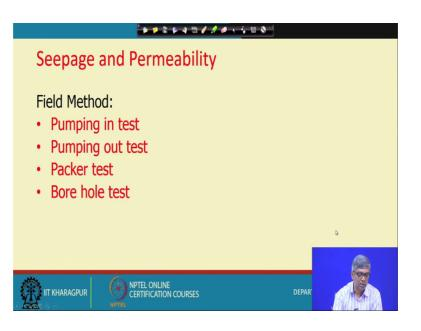
And now I will show you, and if it is a field, there are many methods are available in the field, and then out of that there is a pumping test is quite popular, pumping out pumping in test, then packet test
