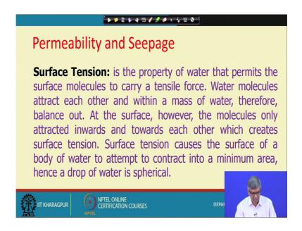
Now, this is the thing which is important for us as I have told you that this is a property of water this surface tension. Capillary is the effect of the surface tension. Capillary is the action and surface tension is the course actually. Whatever I have said that if the voids are fine and water will be raised; how it will be raised? Because of this capillarity and capillarity caused by what? Surface tension. So, this is the thing.
