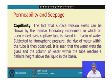
Then capillarity; the capillarity is an action, the fact that surface tension exist can be shown by the similar laboratory experiment in which an open ended glass capillary tube is placed in a basin of water. So, in a basin of water if I put a very fine tube on the water both side open, subjected to atmospheric pressure, the rise of water within the tube is then observed
