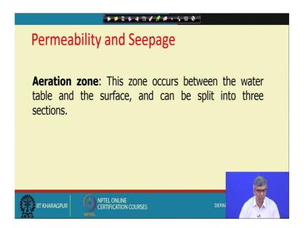
And then saturation zone I have divided actually wanted to divide into 2 parts; one I have already explained, it is saturation zone and other one, aeration zone. This zone occurs between the water table and the surface and again this can be split into 3 distinct zone, section.
