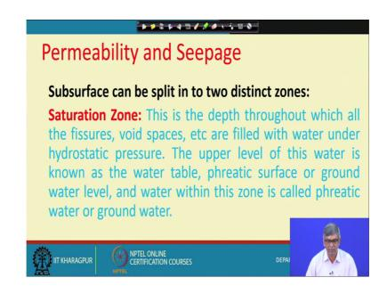
And, then subsurface can be split into 2 distinct zone; one is saturation zone, by the name itself it is quite clear and obvious that saturation means all soil mass, will have a voids and all void spaces will be filled up with water. This is the depth throughout which all the fissures, void spaces, etcetera are filled with water under hydrostatic pressure. The upper level of this water is known as the water table and phreatic or sometime it is known as phreatic surface,
