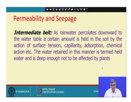
And then intermediate belt; that means, capillary fringe means what? it was not below water table above water table, but because of this capillary action some water will be raised up and water and soil will be saturated. So, that is called capillary fringe and intermediate belt is what? As rainwater percolates downward to the water table a certain amount of water is held in the soil by the action of surface tension, capillarity, absorption, chemical action etcetera.
