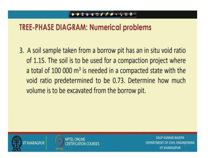
Next problem suppose, third problem again similar a soil sample taken from a borrow pit has an in situ void ratio of 1.15 the soil is to be used for a compaction project where a total of 100 1000 meter cube is needed in a compact it is a state with the void ratio predetermined to be .73, determine how much volume is to be excavated from the borrow pit.
