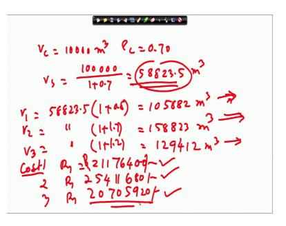
So, for these let us do, you know that actually construction site V S was 100 1000 meter cube and your ec equal to 0.7 and then I can find out from here V S equal to 100 1000 divided by 1 plus 0.7 so that gives you 58823.5 meter cube. That means out of 100 1000 meter cube of soil compacted soil, the solid will be this much and this amount of solid should be there in each of the sites.
