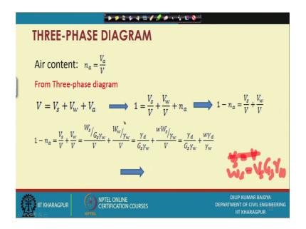
Now, air content; air content actually is defined as na, and which is by definition Va by total volume; that means, with respect to total volume, how much volume of air is present. So, you can, as we have done that three phase diagram, the total v can be expressed into Vs plus Vw plus Va, and this one if I divide it by Va if I divide it by V everywhere, and you can see this side this become 1 Vs by V Vw by V and this will become Va by V. So, this is n na.
