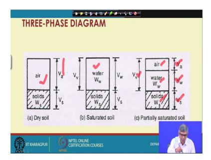
And now I have shown in the previous diagram only two phase diagram, because only I have considered voids only, and we have considered solid, but if I consider void is completely dry, then this is the diagram we can think of. This is the diagram we can think of; that is dry condition only air, and only solid and if the all the voids filled up with water; that means, saturated then I can think of, this is the diagram; that means, this is the volume of water and this is the value of solid.
