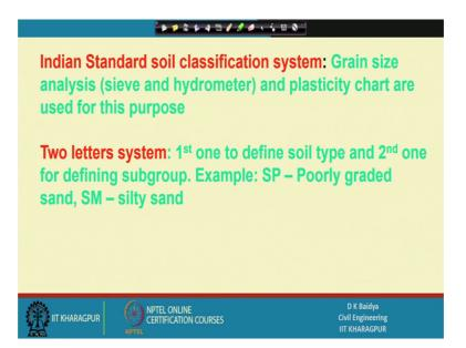
First one define the soil type and second letter defining subgroup an example is like this sp an one soil is classified finally, as sp what it means it means poorly graded sand.
