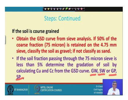
So, that is the thing to be considered and next step is if the soil is coarse grained suppose if it is more than 50 percent retained by 75 micron, then you have decide it is a coarse grained then coarse grained soil if it is coarse grained immediately what is your next action next action will be after in the GSD means grain size distribution curve from sieve analysis.
