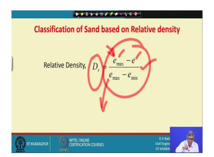
and next is when there is a granular soil, then sometime granular soil can be classified another way that is by relative density and what is the relative density the expression for relative density is given here this expression is given of relative density and relative density universally it is used a notation Dr and that expression Dr related equal to e max minus e divided by e max minus e minimum.
