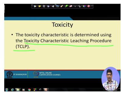
So toxicity characteristic which we said that we will try to explain a little bit more further, this toxicity characteristic is determined by a test which is known as the toxicity characteristic leaching procedure. And this test is one of the highly used and I would say highly abused test in waste management system.
