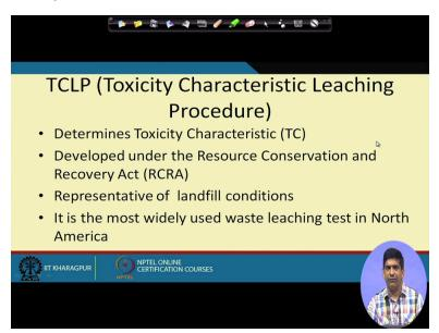
So in terms of the TCLP test which we are talking about, it is determines the toxicity characteristics, it finds out the toxicity characteristics of the waste. It was developed by US EPA under RCRA which is Resource Conservation and Recovery Act. And what it does? It represents
