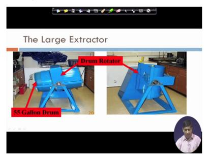
So here we had a large extractor which is a 55 gallon drum and be put it in there then we had the rotation. In terms of the rotation it was half of the TCLP standard TCLP rotation, because of a big drum it was difficult to rotate at 32 rpm it was at 16 rpm. So the testing was done to compare how the big compares with the small in terms of sorry how the rpm speed has an impact.
