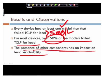
So what was found? It was found that every device had at least one model that failed TCLP for lead. So when we say failed TCLP, what do we mean? We mean that the concentration of lead in the fluid in the liquid that after rotation we take the liquid sample, so filter it through 0.45 0.7 micron and then take the liquid sample and then digests that sample and tested it on
