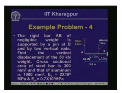
Now we have another problem which is a similar type but of little variation that the rigid bar AB of negligible weight is supported by a pin at B and by two vertical rods of aluminum and steel; we will have to find out the vertical displacement of the 50 kilo Newton weight at this location, how much displacement it undergoes etc, the parameters of these members are given.
