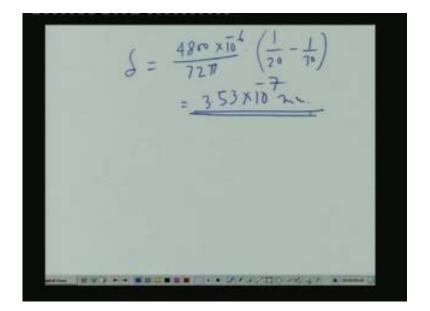
If we compute the whole thing it is 4800(10 to the power minus 6) by 72pi (1 by 20 minus 1 by 30 is equal to 3.53(10 to the power minus 7). This is the value of the delta which we get from the competition for the value of the delta for the varying diameter.
