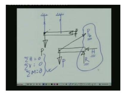
This is connected by two wires of this particular form. Now these rods will undergo extension because they are subjected to axial pull when this particular load will be acting.
