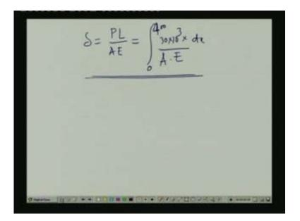
So we compute delta is equal to P L by A E now, here this bar is undergoing an axial pull with a load of 30 kilo Newton so we have restricted this over the length L which is 0 to 400 P is 30 kilo Newton. Since we are taking the diameter of small segment which is dx so A is a function of x and we have a value of E. This if we integrate then we get the extension of the bar.
