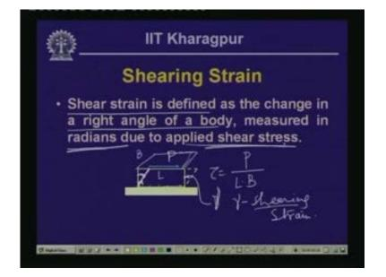
Now having looked into the strength in the axial direction when it is acting only in one direction or acting in the two directions, where in we have the strains  $epsilon_x epsilon_y$ . We discussed the stresses we encounter, the stress which is in the x direction in the y direction and also the body undergoes at a point a stress which we call as a shearing stress which acts between the two planes.
