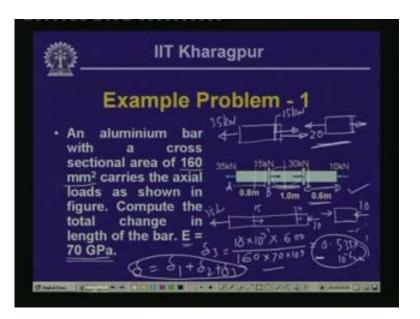
Here are some example problems based on the aspects discussed earlier. An aluminium bar which is having a cross sectional area of 160 mm square carries the axial load as shown over here. We will have to compute the total change in length of the bar and the modulus of elasticity E is given as 70 GPa the Gigapascal.
