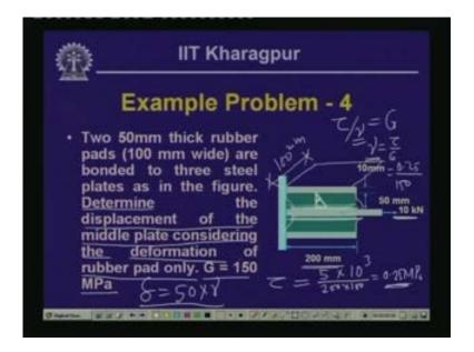
I have another problem which is the applications of the concept of shearing strain. There are 2 rubber pairs, there are 3 steel plates of 10 mm thickness and 2 rubber pairs are attached to this steel plates in between the steel plates which is of the rubber pair
