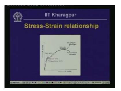
If you can remember last time I had demonstrated that the stress strain relation ship is of this particular form where this axis represents strain and the y axis represents stress. Now, say that if we keep on applying load on a bar in an axial manner if we apply a tensile pull to a bar gradually, the bar will undergo deformism and thereby you exceed that for a bar which is subjected to axial pull how to compute the strain corresponding to that port each increment of the load.
