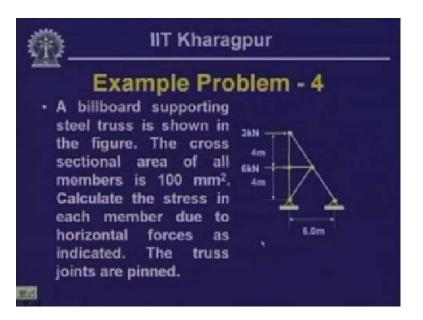
Here is another problem, this is the supporting structure which supports a billboard, many a times we use boards, sign boards on which the advertisements are put and these boards are supported by some steel structures and these boards are subjected to the wind pressure.
