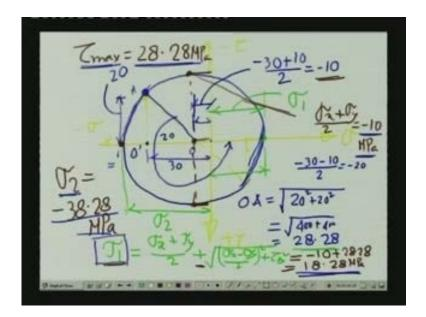
We can evaluate the position of these planes, the maximum, and minimum normal stresses with reference to the plane. Now this is the plane which is representing the vertical plane, normal to the plane which coincides with the x-axis, which you call as x-plane.
