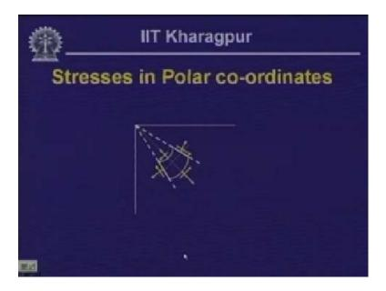
Here I have tried to represent state of stress at a particular point in a stress body, and as we have designated that this particular stress which is acting normal to the r-plane, let us call that as  $\sigma_r$ . Let us assume that this particular distance is dr. The first radial line let us call, this is at distance of  $\theta$ , and the small angle made by these two radial line is d $\theta$ . The radial distance from the origin to the first part of the element, let us call that as r.
