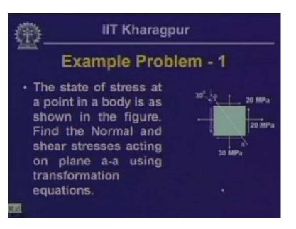
Having known these transformation equations, the concept of the Mohr's circle, and the concept of the octahedral stresses acting on the octahedral planes let us look into some examples on how we compute stresses on any plane if we know the stress at a particular point on a body through the rectangular stress components like  $\sigma_x$ ,  $\sigma_y$  and  $\tau_{xy}$  in two dimensional plane.
