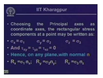
So if we take those components as,  $\sigma_x$  is equal to  $\sigma_1$ ,  $\sigma_y$  is  $\sigma_2$  and  $\sigma z$  as  $\sigma_3$ . The shearing stress components on this are zero because those are the principal planes.
