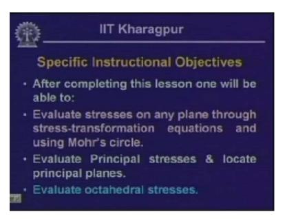
Now, it is expected that once this particular lesson is completed, one should be able to evaluate stresses on any plane through stress transformation equations using Mohr's circle. We will be looking into some more aspects of it then evaluate principal stresses and locate principal planes at a particular point on the stress body. Also, one should be able to evaluate octahedral stresses which we will look into in this lesson.
