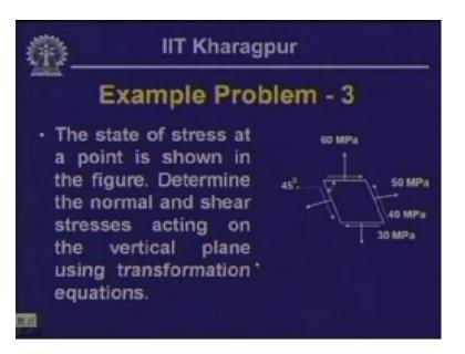
The state of a stress at a particular point is shown in the figure. Determine the normal and the shear stresses acting on the vertical plane using transformation equations.
