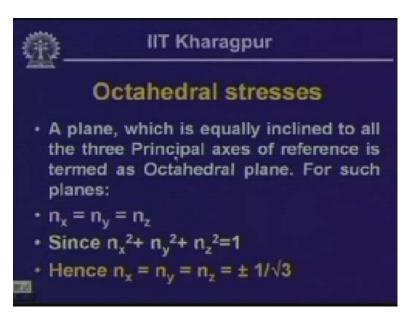
So this is what is indicated here: For octahedral planes which are equally inclined to the reference principal axes, they have the direction cosine of  $n_x$ ,  $n_y$  and  $n_z$  all equal. We have seen earlier that the  $(n_x)$  whole square plus  $(n_y)$  whole square plus  $(n_z)$  whole square the direction cosines of three planes is equal to 1. So there by it leads us to the value of  $n_x$  is equal to  $n_y$  is equal to  $n_z$  as plus or minus square root of 3 of the octahedral planes.
