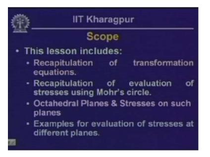
The scope of this particular lesson includes recapitulation of transformation of equations which we have derived earlier, recapitulation of evaluation of stresses using Mohr's circle. We will be looking into some aspects of octahedral stresses; we will define octahedral plane and stresses acting on such planes and then we will be looking into some examples of how to evaluate the stresses at a particular point at a stress body.
