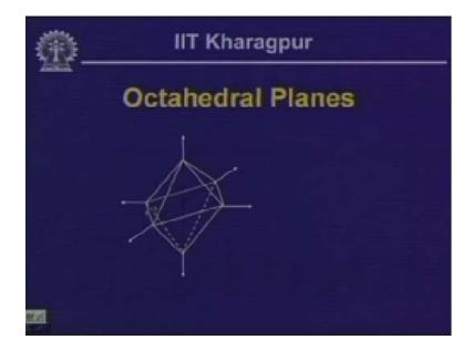
So this is the representation of the octahedral planes, in fact the planes which are equally inclined with reference to the principal axes system, we get eight such planes. This represents  $\sigma_1$ , this is represents  $\sigma_2$  and this is represents  $\sigma_3$ . Now we will get eight such
