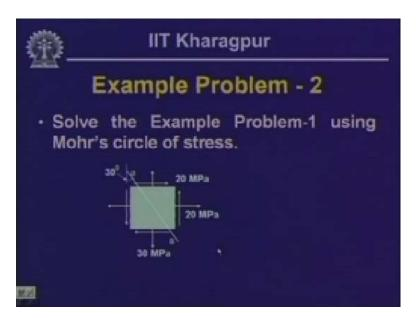
Let us look into this example 2 where we will have to solve this particular problem or rather we have to solve this which is represented in 1 using Mohr's circle of stress. In the previous problem we used the transformation equations for the solution of the stresses at
