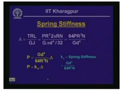
If you remember for the close-coiled helical spring we had the value of the deflection delta because of the action of the axial load P was  $\frac{64PR^3N}{Gd^4}$ , where these terms again;
