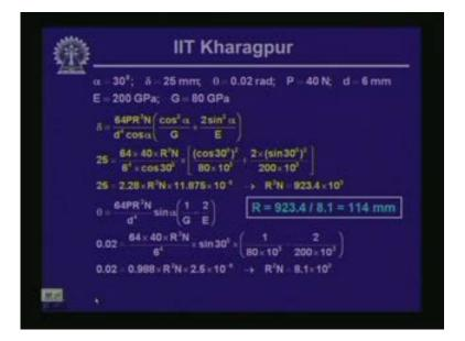
Delta is given as  $\delta = \frac{64PR^3N}{d^4\cos\alpha} \left(\frac{\cos^2\alpha}{G} + \frac{2\sin^2\alpha}{E}\right)$  and since the limiting delta is 25mm, if we substitute the values except this R and N, then we get the value of  $R^3N$  as equals to  $923.4 \times 10^3$ .
