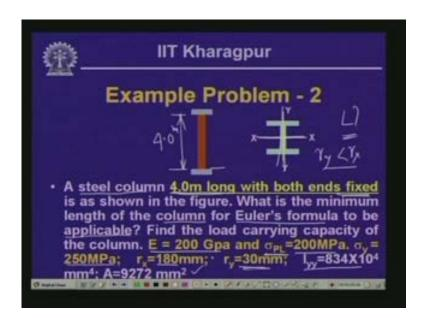
Now the question is let us first find out that what is the value of the limiting length up to which the Euler's critical buckling load formula can be applied.
