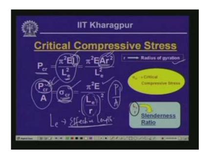
Here you see, from these two expressions we are getting two terms: one we call as the sigma cr the critical compressive stress and another term which is emerging out is the effective length L e by r ratio and this particular ratio we call it as slenderness ratio. It indicates that how slender or how long the member is with reference to its cross-external area. This is what is indicated over here that L e by r is the slenderness ratio and sigma cr is the critical compressive stress.
