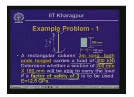
Now let us look into this that if we compute the value of the critical load using Euler's critical buckling load formula see that the value of the I y..... now as I was telling you the cross section is a rectangular one, 150 by 200 and the rectangular access system of this is xx and yy. Now, which can compute the moment of inertia of this section I x and I y?
