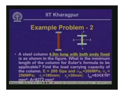
Well, let us look into another example and this particular example is a steel column of length 4m and the ends of this particular column is fixed; both the ends are fixed. Now what is the minimum length of the column for Euler's formula to be applicable?
