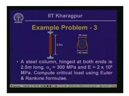
Now let us look in to another example problem wherein this particular member is having a cross section of that of a tube. So it is a tubular member which is subjected to a compressive load and this particular member is hinged at both the ends. That means this is hinged hinged column for which we have seen that P critical is equals to pi square EI over L square and thereby the coefficient K is equals to 1; the effective length coefficient is equal to 1.
