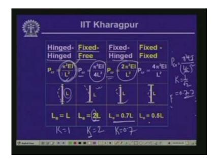
And if we consider a case where the supports are fixed at both ends, the column member is fixed at both ends then the critical load which we get is equals to 4 pi square EI over L square and thereby we can write P cr as equals to pi square EI by L by 2 square and thereby K is equals to half over here and that is what is indicated that effective length is 05 times L so k is equals to 0.5.
