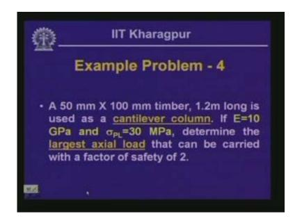
Well, let us look into another example wherein we have a member which is made out of timber, the cross section of which is a 50 mm by 100 mm rectangular one and length of the member is 1.2m. Now this particular member is used as a cantilever column; the value of e is given as 10 GPa 10 Giga Pascal and the stress at the proportionality limit is 30 MPa; we will have to determine the largest axial load that this member can carry with a factor of safety of 2.
