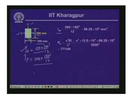
Clearly from this expression you can see that the value of I x should be higher than the I y and as you know that the value of r is equals to root of I by A; and for this particular section we will have two values of r which is r x and r y and r x will be equals to root of I x by the cross-sectional area and r y will be equals to root of I y by the cross-sectional area.
