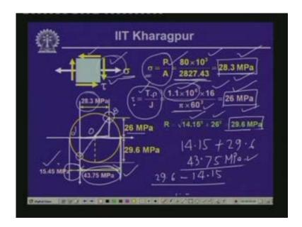
Hence, the maximum tensile stress that is occurring at that particular point is 43.75 Mpa, the maximum compressive stress that is occurring is 15.45 Mpa and the maximum value of the shearing stress, the in-plane shearing stress that is occurring which is the radius of the Mohr's circle is equals to 29.6 MPa; these are the values which we wanted to have.
