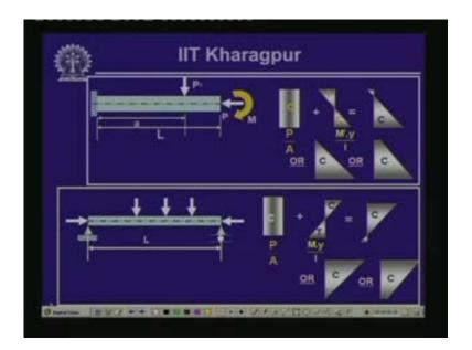
Now we had looked into in the last lesson that there could be cases with reference to either a cantilever beam or simply supported beam or for that matter any of such members where it is supported at suitable supports and is subjected to axial load as well as the transverse load.
