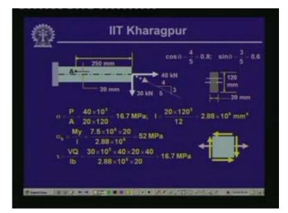
Now this is what is indicated over here. First thing is that we have decomposed this inclined load which is at an angle of theta in two directions: one in the axial direction,
