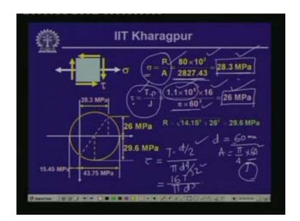
We get a normal stress of 28.3 Mpa and shearing stress of 26 Mpa. Now if we plot these stresses in the Mohr's circle and the values or the directions are shown over here; sigma being a tensile stress is positive and tau here is giving shearing stress which is in the negative direction.
