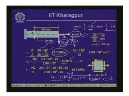
So these two stresses since they are of the same nature because they are tensile we can add them together. The normal stress because of the bending is equals My by I and as we have seen here M is equals to 7.5 kilonewton per meter into 10 to the power 6 will give you Newton millimeter times y, y is 20 because point A is located at 20 mm away from the neutral axis and I is equals to 2.88 into 10 to the power 6 which is b h cube by 12.
