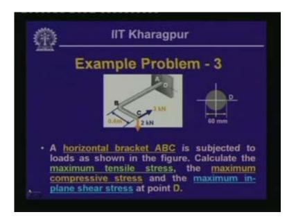
Well, let us look into another interesting problem where this is a horizontal bracket A b and C, it is in the horizontal plane; now this is subjected to a load at the tip; one is a vertical one which is of magnitude 2 kilonewton and another one we have a load which is 3 kilonewton which is acting parallel to the arm AB. Now what we need to do is that we need to compute the value of the stresses at a point D which is at the support which is at A.
