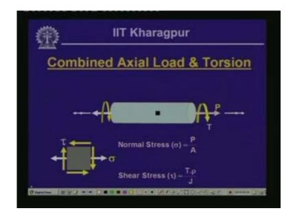
In the last lesson we had looked into some numerical example where a member was subjected to the axial load and the transverse load which was causing bending in the member, thereby the member was under the action of axial load and the bending. Now in this particular case we are going to consider that if a member is subjected to the axial load and a twisting moment then what happens to the combined action of this loading.
