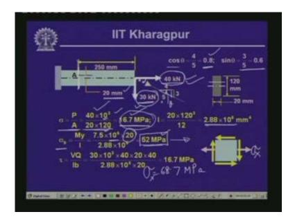
Now, in the y directions we do not have any normal stress so that is 0. The shear force which we have seen as V equals to minus 30 kilonewton will produce the shearing stress at this particular section A which is equals to VQ by Ib and V is 30 into 10 to the power 3; now Q is the first moment of area of the cross section above the section where we are computing the stress.
