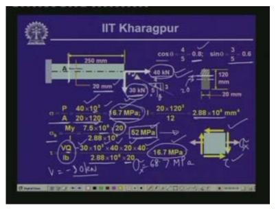
This is the state of stress that we have at that particular point A wherein we have the normal stress sigma x and the shearing stress tau. Now as you know that at a particular point when we have the combination of the normal stress and the shearing stress we can calculate the value of the maximum normal stresses and the maximum shearing stresses using the transformation equation or using the Mohr's circle.
