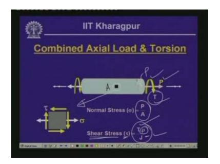
Therefore, if we look into this particular element this element will be subjected to the shearing action because there is a twisting moment which is a positive twisting moment, on this element (Refer Slide Time: 16:06) we will have the shear which will be acting on this form and that is what is represented over here which is resulted from this twisting moment T and these are the complementary shear because of this shear and sigma is the normal stress that is acting.
