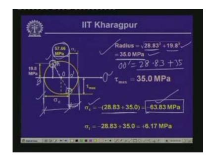
Hence, at the member, at that particular point here the magnitude of the maximum compressive stress is 63.83 MPa and 6.17 is the 6.17 MPa is the maximum tensile stress. Now the value of the maximum shearing stress in-plane shearing stress if you
