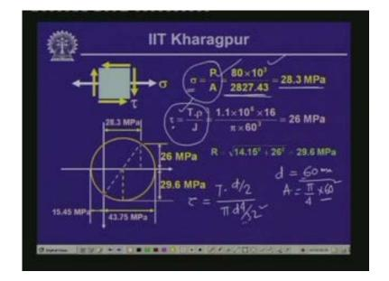
As you know that polar moment of inertia for the circular section is pi d 4 by 32 and rho is the maximum distance from the center which is d by 2 over here so we are going to get the maximum shearing stress which is d by 2. So, eventually this gives us 16 T by pi d cube.
