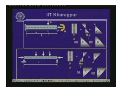
Now if we idealize the particular situation then probably we can describe the same thing in this particular form that we have a cantilever member which is fixed at one end and free at the other and at this end we have a concentrated load P which is acting through the center of this particular member along with moment M bending moment M and we have a transverse load P which is acting at a distance of a from the support.
