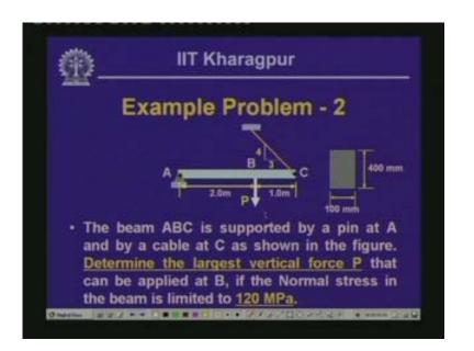
Now let us look into another example where we have a beam which is simply supported the beam A B C is supported by a beam at A and by a cable at C at this point (Refer Slide Time: 51:32). Now what you will need to do is you will have to determine the largest value of P so that the normal stress in the beam is limited to 120 MP a. If the normal stress value is 120 MPa then what will be the value of P? The cross section of the beam is 100 by 400.
