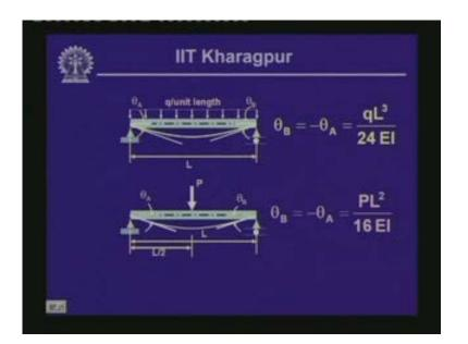
Here if you look in to, see the values of the end slopes as we have computed for these two different cases when the beam is subjected to uniformly distributed load of magnitude Q per unit length we have computed the value of theta B and theta A and we have seen the magnitude is qL cube by 24EI. Now if the same simply supported beam if it is subjected to a concentrated load at the center the value of the end slope comes as PL square by 16EI.
