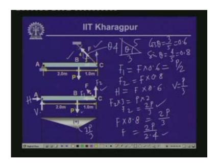
Now physically if you look into, because of this load P at the top you will get compressive stress and at the bottom you will get tensile stress. Now if we combine the compressive stresses because of the axial compression and the bending you will get the maximum compressive stress and if that will limit to 120 then we will get the value of the maximum stress.
