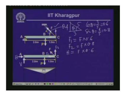
Now if you take the moment of the forces with respect to A, we have F 2 into three is equals to P into 2 and thereby F 2 is equals to 2 P by 3. Now F 2 we have seen is equals to F into 0.8 so F into 0.8 is equals to 2 P by 3 or F is equals to 2 P by 2.4. If this is F then the vertical force F 2 we have got as 2 P by 3 and F 2 plus V will give you P so V is equals to P by 3.
