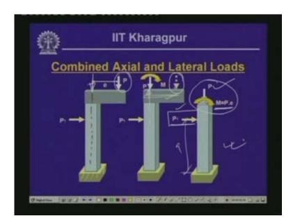
Now if you remove this vertical bar I mean this horizontal member then the vertical bar we have the effect of this eccentric load as a load P which is concentric now which is acting through the cg of the member and we have a moment which is equal to P times e where e is the eccentricity or the distance of the cg from this loading point. Also, this particular member is subjected to concentrated load P 1 which is acting at a distance let us say A from the support.
