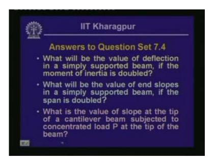
Well, let us then look into the answers to the questions which were posed last time. The first question was what will be the value of deflection in a simply supported beam which is simply a supported beam if the moment of inertia is double.
