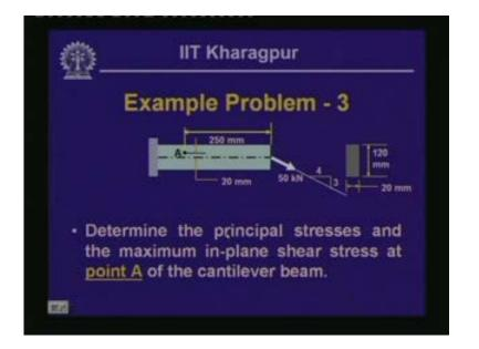
Well, we have another example problem that you need to determine the principle stresses and the maximum in-plane shear stress at point A which is at a distance of 20 mm from the centroidal axis and it is subjected to load of 50 kilonewton acting at the center of the beam in an inclined form and you look into this problem and we will discuss about this in the next lesson.
