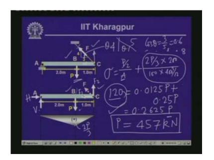
So you see that we can compute the maximum value of load P which can be applied here so that the stress does not go beyond 120 and here we get the combined actions of this axial stress as well as the bending stress.
