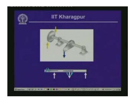
Now this is another case wherein we get the values of the loading in combined form. Let us say this is a shaft and this particular shaft is subjected to or is attached with a gear where we have a couple which is giving a twisting movement in the shaft. Also, if you look into this particular shaft it is having a member which is extensive with respect to the shaft center line and there is a concentrated load acting at the end of this particular member.
