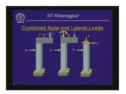
Well, now let us look into a case where we get a combined loading form wherein we have a vertical member which is fixed at the base and at the top we have a rigid bar on which a load P is acting which is eccentric with respect to the center line of this member or the cg of this vertical member.
