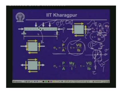
Here you can see that the sigma is equals to P by A on this particular element and consequently we have tau equals to VQ by Ib and incidentally the shearing stress at this particular location will be maximum as we have seen. Again we will have the normal stress sigma and the shearing stress tau and based on these values we can compute the value of maximum principle stresses.
