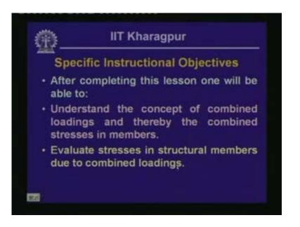
Hence, once this particular lesson is completed one should be in a position to understand the concept of combined loadings and thereby the combined stresses in members. Also, one should be in a position to evaluate stresses in structural members that are developed due to such combined loadings.
