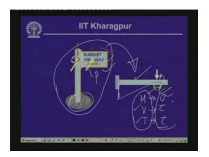
Thus, you see that this particular member is subjected to the action of bending moment, shear force and the twisting movement and thereby we will have the resulting normal stress and the shearing stresses or each individual load we can compute the values of the normal stress and the shearing stresses and once we know the values of the normal stress and the shearing stress then we can compute the resultant stress in terms of the normal stress and the shearing stress.
