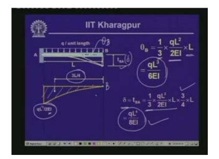
Therefore, by employing moment-area method to this we can compute the value of the slope and the deflection of this particular beam.
