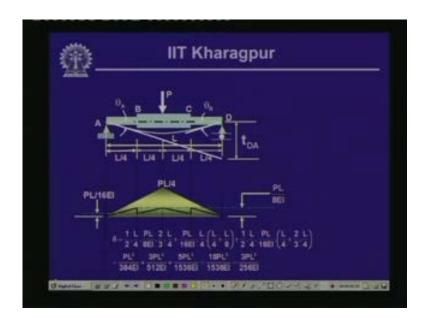
Now here as you can see that the maximum value of the bending moment is PL by 4 at the center which is P by 2 times L by 2 and at this point the value of the bending moment is P by 2 times L by 4 which is PL by 8 and so is at this point as PL by 8.
