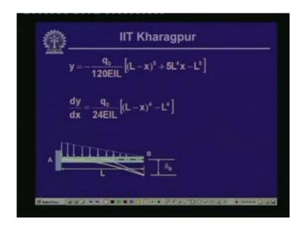
And if you substitute x as equals to L you get the value of y at the tip and dy dx at the tip. Now x equals to L means this goes off so you have 5L to the power 4, L to the power 5 minus L to the power 4 so this becomes q0 by 30 q0 L4 by 30EI that is the value of the deflection which is again negative so it is downwards and at x equals to L if you compute this you get minus q0 L cube by 24EI as the slope of this particular free end. (Refer Slide Time: 56:18)
