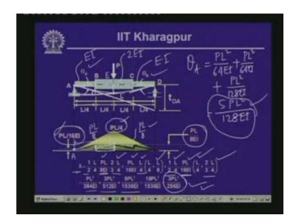
Now if we again make a comparison of the values which we have seen earlier, now in a simply supported beam where the value of the moment of inertia is uniform right through where the flexural rigidity is uniform then we have seen the value of the maximum deflection is PL cube by 48EI and the values of the slope as PL square by 16EI.
