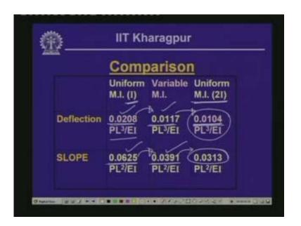
Therefore, by making variable moment of inertia in fact we can achieve economy both in terms of the deflection or the stresses and as well as the economization on the uses of the material and thereby where we have the larger value of the bending moment if we go for a larger cross-sectional area thereby you can have less stress, you can have less deflection, you can have less values of the rotation at the end.
