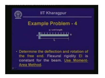
Well, we have another example where it is a cantilever beam subjected to uniformly distributed load and the flexural rigidity EI is constant for the beam; you will have to use moment-area method.
