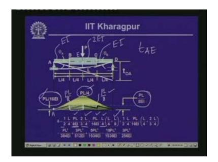
And thirdly, we have this triangular area which is half times L by 4 is the length, PL by 16EI this is PL by 8EI is the total ordinate minus PL by 16EI so balance is PL by 16EI and the moment of this c g from moment of this particular area with reference to this distance is L by 4 plus two third of L by 4.
