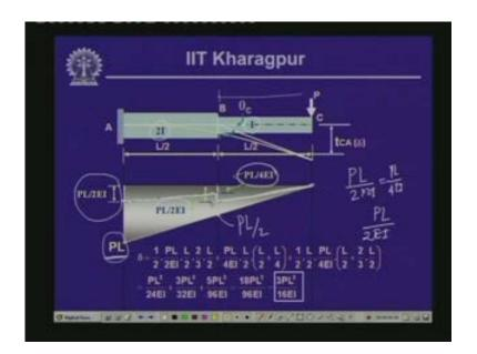
Now we will have to employ this M by EI diagram to compute the value of the slope and the deflection. Now for computing the deflection of the slope what we need is now we need to use the moment-area method and for using moment-area method we will have to employ the moment-area theorems and as you know that for employing moment-area theorems we will have to deal with the M by EI diagram.
