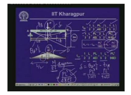
Now what will be the value of rotation over here; as we have seen that theta A equals to PL square by 16EI. Now if we draw a tangent at this particular point at the center point of this beam that becomes..... now if we draw the tangent at this particular point of the elastic curve the tangent at this point is horizontal and as we exceed this gives us the maximum value of the displacement or the deflection where the tangent to the elastic curve is horizontal.
