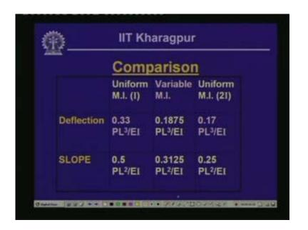
Consequently, if we make the value of I as 2I right through that means if we have uniform flexural rigidity but instead of EI now it is twice EI that means we are adding more material to it then naturally the values of the deflection will be half of the previous one and so will be the slopes.
