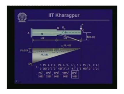
This is the bending moment diagram that means zero bending moment over here and at this point we have the maximum value of the bending moment which is equals to PL. So this external one shows the bending moment diagram which is varying from 0 to linearly from 0 to PL.
