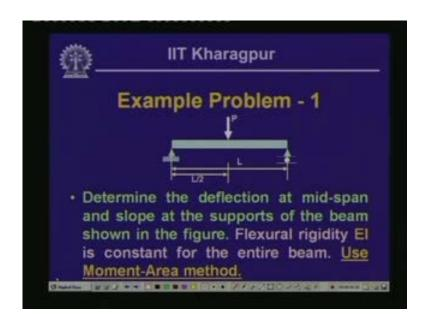
Well, let us look into the example problem which I had given to you last time for evaluating the slope and the deflection so the deflection at the mid-span and slope at the supports for loading indicated over here. And we will have to use moment-area method to evaluate the slope and deflection.
