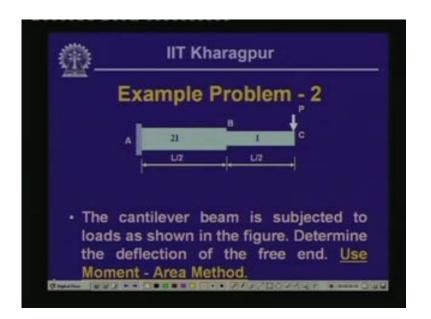
Well, now let us consider an example where the moment of inertia is not constant throughout the beam instead we have variable moment of inertia. Over the part AB we have the moment of inertia as 2I and over the part BC the moment of inertia is I.
