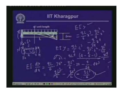
So dy dx at x equal to L is minus qL cube by 6EI dy dx is equal to minus qL cube by 6EI. This is the value of the slope at the free end and the deflection at the free end is equal to qL 4 by 8EI.
