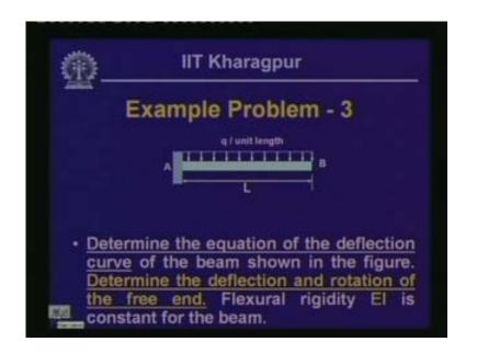
So we can adopt either EI d 2 y d x 2 equal to moment or EI d 4 y dx 4 equal to the minus of the loading. now let us look into another example where this is a beam; now this is a different type of beam, the beam is fixed in a and is free at the end b and thereby as we know that this is a cantilever beam and this beam is subjected to uniformly distributed load of q bar unit length.
