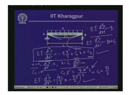
Now if we substitute that x equal to 0 d 2 y dx equal to 0 this gives us that C 2 is equal to 0. now if we substitute this that at x equal to L d 2 y dx 2 equal to 0 we get C 1 into L is equal to qx square by 2 and x is L so this is L square by 2 so L square gets cancelled so this gives us that C 1 is equal to qL by 2. Hence the expression here that we get EI d 2 y dx 2 this is equal to qL by 2 x minus qx square by 2.
