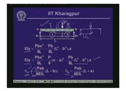
Now, if we substitute the values of b and a as L by 2 then we get the expressions like this that when the load P is acting at the center of the beam thereby a is equal to L by 2 and b is equal to L by 2.
