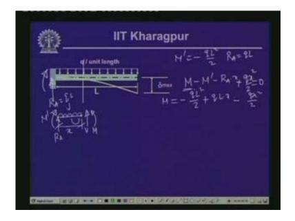
Now if I substitute the value of the moment in the differential equation so we have EI d 2 y dx 2 is equal to moment which is qL x minus qL square by 2 minus qx square by 2. Now if I integrate this we have EI dy dx this is equal to qL into x square by 2 minus qL square by 2 x minus q by 2 into x cube by 3 plus you will have the constant C 1.
