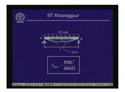
Now last time we had evaluated the expression for the elastic curve and subsequently the deflection at different points. Now what is the simply supported beam when the load is w for unit length along the entire span or what is the entire length of the beam?
