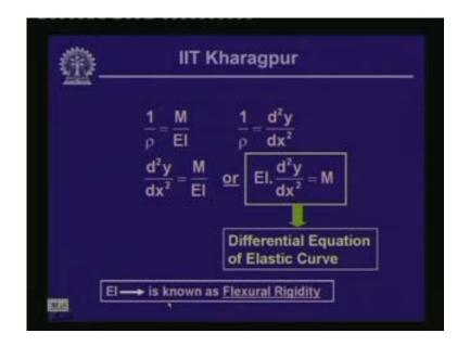
Now, if you remember, last time we had derived that if a beam is subjected to transverse loading then it undergoes bending and therefore the axis of the beam if you look into it deforms. And we have seen that in terms of curvature of this particular beam 1 by rho is called as curvature which you can write as d 2 y dx 2 where y is the deflection of the beam with respective is Avenal position.
