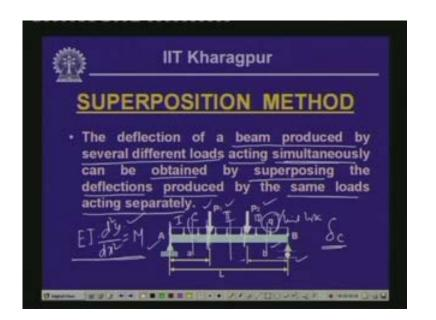
Also we can compute the value and accordingly at y we can compute from this expression for y which will get as a function of x so at a distance from here if we know this value of x we can compute the value of y. Now also what we can do is we can compute the value of delta c by taking these loads acting individually.
