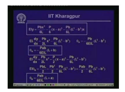
It is that EIy is equal to Pbx cube by 6L minus p by 6(x minus a) cube minus Pb by 6L (L square minus b square) x. This is the value of C 2 this is for the second part and for the other part we substitute the value of C 1 and we get the expression for EIy.
