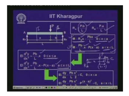
Now, once we integrate these expressions we come up with this that EI dy dx is equal to Pb by L; now x will give us x squared by 2 by two with the constant of integration C 1 and again the validity is between 0 to a.
