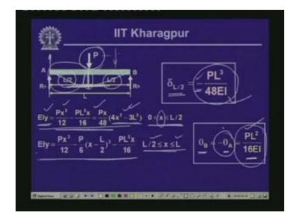
So, when we talk about a particular case then delta maximum is PL cube by 48 EI and theta a equal to theta b magnitude y that is PL square by 16 El.
