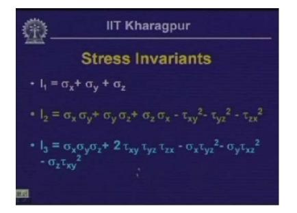
That is why these coefficients  $I_1$ ,  $I_2$  and  $I_3$  are known as stress invariants. Let us see how to solve these stresses in some physical problems? In this particular example here there are two plates which are connected together by a bolt and it is subjected to a pull - external force P. This is the plan of the two plates and if we take a section we cut the plate here and cut the plate here and view from this side then the section looks like this.
