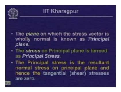
Now the plane on which this stress vector is fully normal is known as principal plane. This is what we considered in the previous situation where we had taken the arbitrary plane and we considered the stress vector which is along the normal and thereby we obtained the cubical equations in sigma<sub>n</sub> and from which we obtained the three roots sigma sigma<sub>1</sub>, sigma<sub>2</sub> and sigma<sub>3</sub>.
