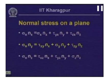
This is what is represented here the equations of equilibrium in the three directions x, y, and z. Now these equations can be rearranged and can be written as  $(sigma_x minus sigma_n) n_x$  plus  $tau_{yx} n_y$  plus  $tau_{zx} n_z$  is equal to 0;  $tau_{xy} n_x$  plus  $(sigma_y minus sigma_n) n_y$  plus  $tau_{zy} n_z$  is equal to 0;  $tau_{xz} n_x$  plus  $tau_{yz} n_y$  p
