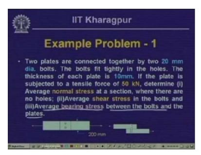
And if we look into the transmission of the force in little greater detail we will see that this is the plate, here two bolts are present and this plate is being pulled by force P. Now the transfer of force from the plate to the bolts which are here when plate is being pulled, this part of the plate, this is the bolt, the hub part of this particular plate comes in contact with this particular bolt and there may be release in the contact between the plate and the bolt surface.
