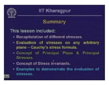
To summarize what we have learnt in this particular lesson; first we recapitulated on different kinds of stresses and those stresses are the normal stress, and the normal stress on an axially loaded bar. What is the maximum normal stress that acts on an axially loaded bar is the axial pull P or compressive force push by cross sectional area and cross sectional area which is minimum is normal to the axis of the bar.
