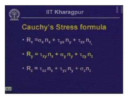
So Cauchy's stress formula is  $R_x$  is equal to sigma<sub>x</sub>  $n_x$  plus tau<sub>yx</sub>  $n_y$  plus tau<sub>zx</sub>  $n_z$ ;  $R_y$  is equal to tau<sub>xy</sub>  $n_x$  plus sigma<sub>y</sub>  $n_y$  plus tau<sub>zy</sub>  $n_z$  and Rz is equal to tau<sub>xz</sub>  $n_x$  plus tau<sub>yz</sub>  $n_y$  plus sigma<sub>z</sub>  $n_z$ .
