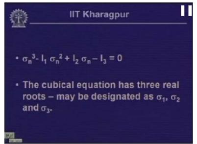
This is the cubical equation in sigma<sub>n</sub>: (sigma<sub>n</sub>) whole cube minus  $l_1$  (sigma<sub>n</sub>) whole square plus  $l_2$  sigma<sub>n</sub> minus  $l_3$  is equal to 0. And once we solve this cubical equation we are expected to get three roots which eventually will turn out be real and we designate those roots as sigma<sub>1</sub>, sigma<sub>2</sub> and sigma<sub>3</sub>. And corresponding to each values of sigma we will get the values of  $n_x$ ,  $n_y$  and  $n_z$ .
