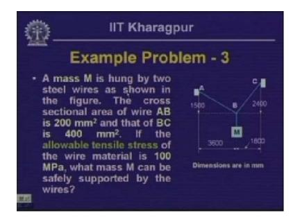
Now in this we have another example problem in which mass is hung by two wires AB and BC and the cross sectional areas of these two wires are given as 200 mm square and 400 mm square. And if the allowable tensile stress of these wire material is limited to 100 MPa then you will have to find out the mass M that can be safely supported by these wires. This particular problem can be solved by taking the free body diagram of this.
