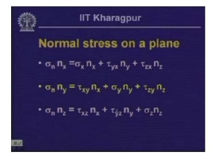
Exactly in the same form the way we have evaluated Cauchy's stress formula taking the equilibrium equations in the x, y and z-direction we can compute the resulting forces in x, y, and z-direction in terms of sigma<sub>n</sub>.
