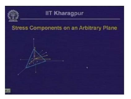
Here are the different stress components that act on any arbitrary plane. Let us consider that A, B, C are any arbitrary plane and o, x, y, and z is the reference axis system. As we have noticed earlier the plane normal to which it coincides with the axis we designate that in the name of the particular axis. Likewise this particular plane is the x plane on which the normal stress sigma<sub>x</sub> acts.
