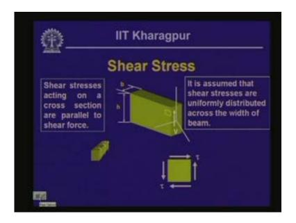
The assumptions are that at any cross section when there is shearing force acting, we assume that the shear stress is parallel to this shear force. That means in this cross section the direction of this shear stress is in the same direction as that of the shear force. Shear stresses acting on a cross section are parallel to the shear force acting in that particular section.
