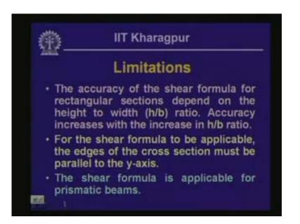
What is the limitation of shear stress formula? While calculating the stresses in a beam due to the shear force we have used the shear formula which is VQ/ib and consequently we calculate the shearing stress at any point along the depth. Now is this particular formula applicable for all kinds of beams or are there certain limitations?
