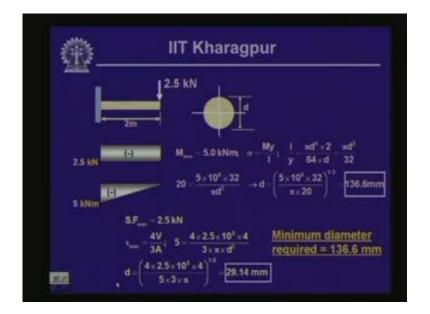
If we draw the bending moment and shear force diagram for this particular pole then the bending moment and shear force diagram is going to be like this, which we have already done earlier. The maximum shear force is going to be 2.5 kN and the maximum bending moment is going to be 5 kilo Nm. Now if we compute the bending stress from this particular expression which is Sigma = My/I and the maximum bending moment is 5 kilo Nm.
