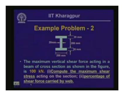
Now we have computed the shearing force, the cross section of the beam and the value of the shear force is known. We have to compute what is the maximum shearing stress that will occur in this particular section and how much shear force is going to be carried by the web out of the total shear force in this particular cross section.
