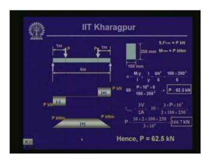
Let us compute the bending moment and shear force diagram. The first step is to evaluate the unknown reactive forces. Let us call this beam as A and B and end A is on hinge so you have a vertical force  $R_A$  and a horizontal force  $H_A$  and the vertical force at B as  $R_B$  as the reactive forces. The summation of horizontal forces = 0 will give you  $H_A = 0$  and you can compute the value of  $R_A$  and  $R_B$ .
