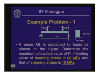
Let us look at some examples I had given you in the last lesson. The beam is subjected to loads P as shown over here where it is a two point loading and they are placed equidistant from the two sides at the distance of 1 meter. Now you will have to determine the maximum allowable value of P if the limiting value of bending stress is 60 MPa and the limiting value of shearing stress is 10 MPa and the cross section of the beam is a rectangular one.
