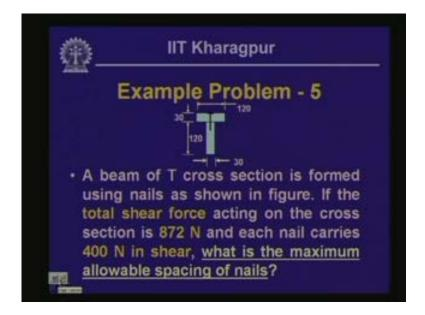
Another problem which is again the cross section of beam is just like a T. Here two rectangular components are there. One rectangle is on the top, one is at the bottom and these two rectangular sections are interconnected along the length using nails and these nails are spaced. We will have to find out the particular spacing so that we know the shearing capacity of these bolts.
