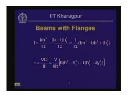
Well these are the values of i of the cross section which is bh to the power of 3/12 for the whole section - the 2 sides of it  $(b-t)h_1$  to the power of 3/12. So this is the value of the moment of inertia I and thereby the shearing stress t and this is the Q of the section above the neutral axis and this is the value of the shearing stress that we are going to get and since  $y_1$  varies we get the variation from the bottom part to the top part.
