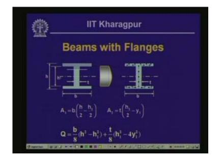
Take another type of cross section where the cross section of the beam is similar to that of 'I'. If you remember while discussing the bending stress, we have discussed that if we take a beam and if we have two rectangular sections placed at a distance apart, then that contributes more to the value of the moment of inertia and thereby we get maximum effect in the bending stresses.
