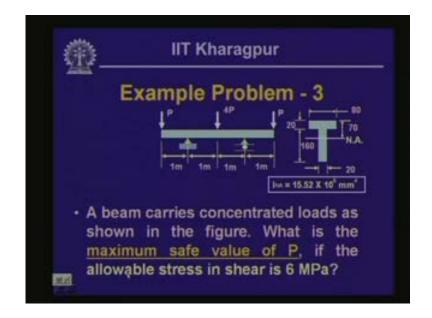
Now let us look into another example where we have a beam and is loaded in this particular form and the loads are P at the two ends and 4P at the center .Now this particular beam is hind at this particular end, let us call this as A, and this end as B ,this point as C ,this D, and this E, so it is hinged at B, and roller support at D, over hang between B and A, and D and E ,and this the loading it has on the cross section. If this beam here is similar to that of T section.
