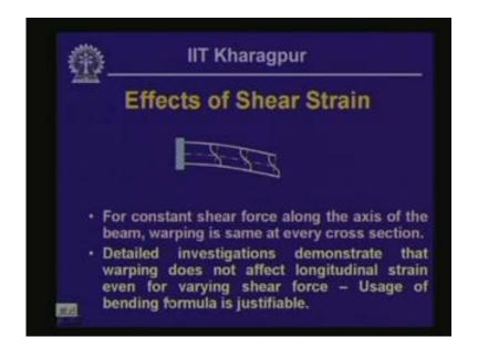
Let us see what the effect of the shearing strain on the longitudinal strain is. Let us consider a cantilever beam whose cross section is rectangular. The shear stress in such a section varies parabolically and since the shear stress Tao varies parabolically the shearing strain gamma which is Tao/G also varies parabolically. So, at the neutral axis we get a shearing strain and since the stress at that neutral axis is higher, the corresponding shearing strain is also high.
